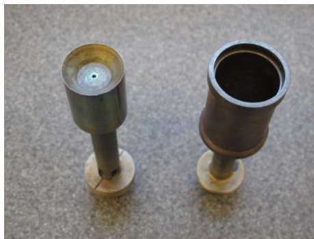
Figure 2: ARES Couette Fixture components. Spindle (left) and Cup (right).
