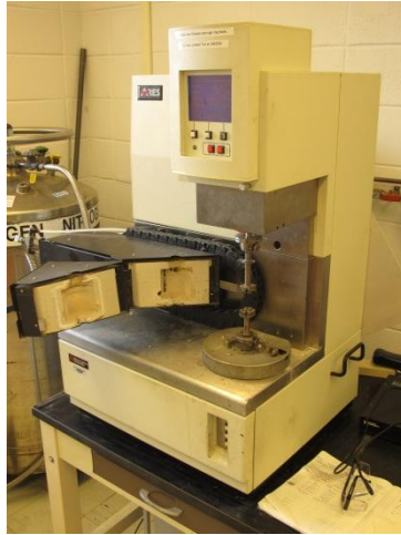
Figure 1: ARES Rheometer mounted with couette fixture and open furnace door.
