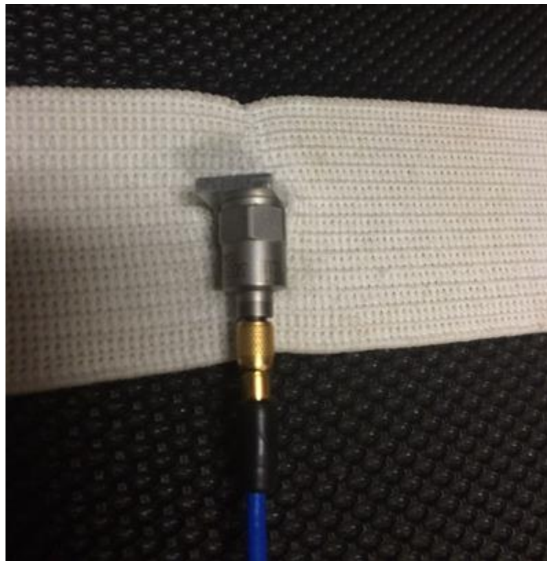
Figure 1 Accelerometer mounted to the holder
