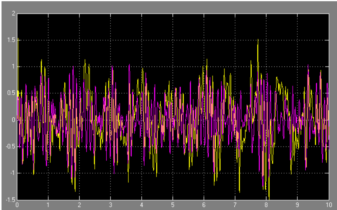
Figure 52 - New algorithm active suspension system output acceleration time response with the input of white noise signal, and compare with passive suspension system
