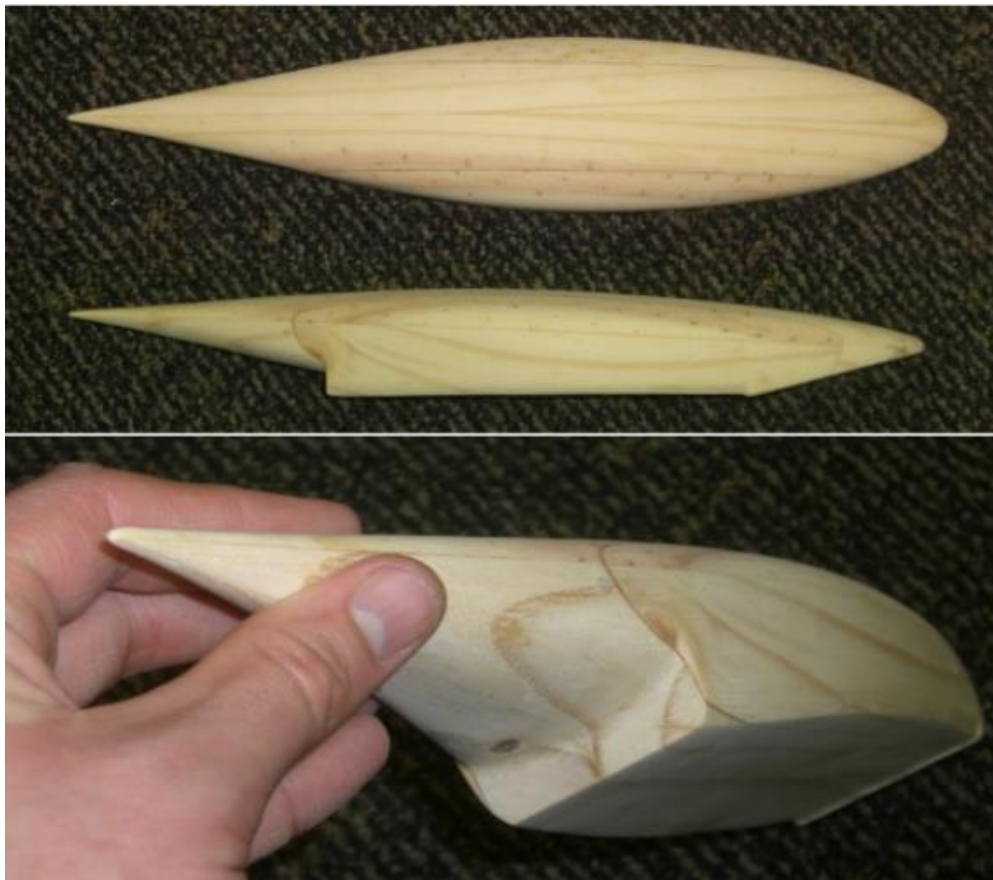
Figure 1: Sponson A: designed to have no aerodynamic lift and low aerodynamic drag, yet good hydrodynamic performance.
