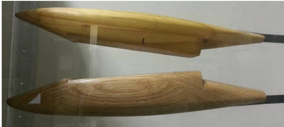
Figure A2: Sponson A (top) and its mirror image (bottom). Only the top model was mounted to the force balance.
