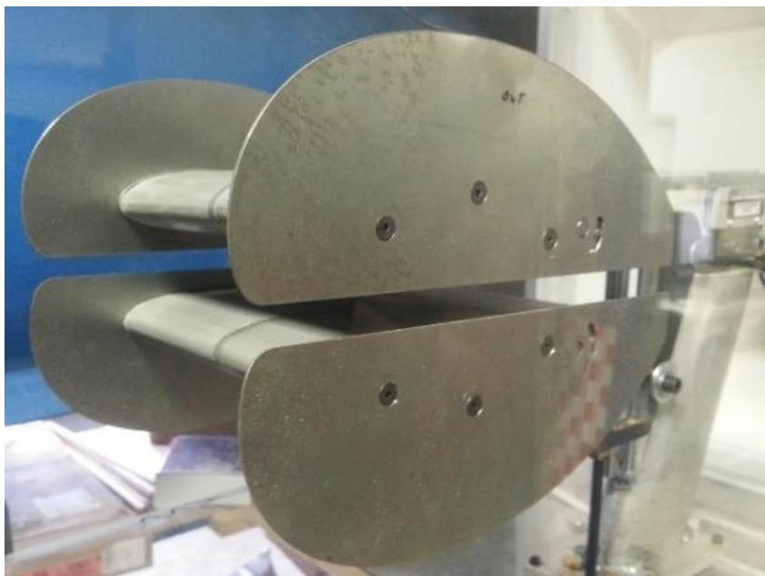
Figure A3: Sponson B (top) and its mirror image (bottom). Only the top model was mounted to the force balance.
