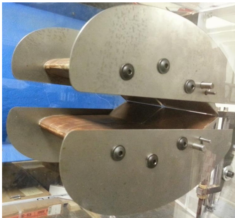
Figure A4: Sponson B (top) and its mirror image (bottom) with end plates and flaps deflected down 30° from original chord line
