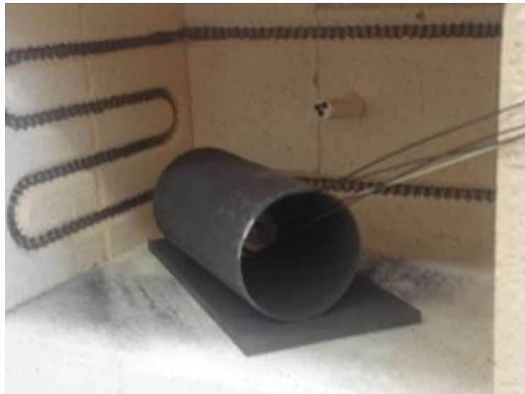
Figure 2. The EPCM in a carbon steel cylinder during heating
