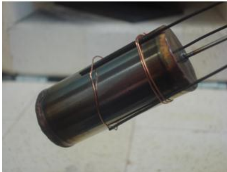
Figure 3. Three thermocouples secured around sample using copper wire
