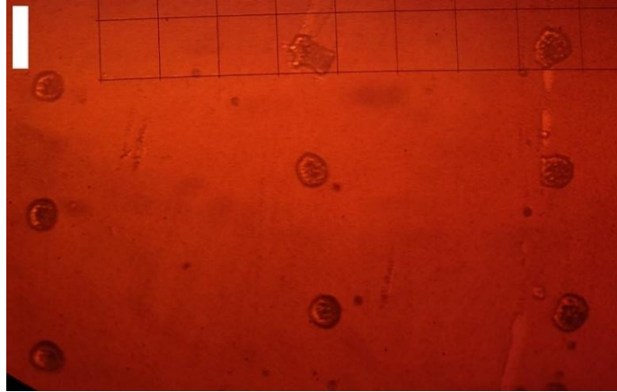
Figure 3.6 Dot matrix on a superhydrophobic surface, scale bar = 0.1mm, grid on the top: 0.1mm × 0.1mm
