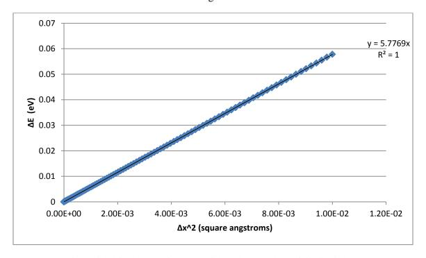
Fig 4. Nickel fundamental frequency trial results. The slope of this line is k/2.
