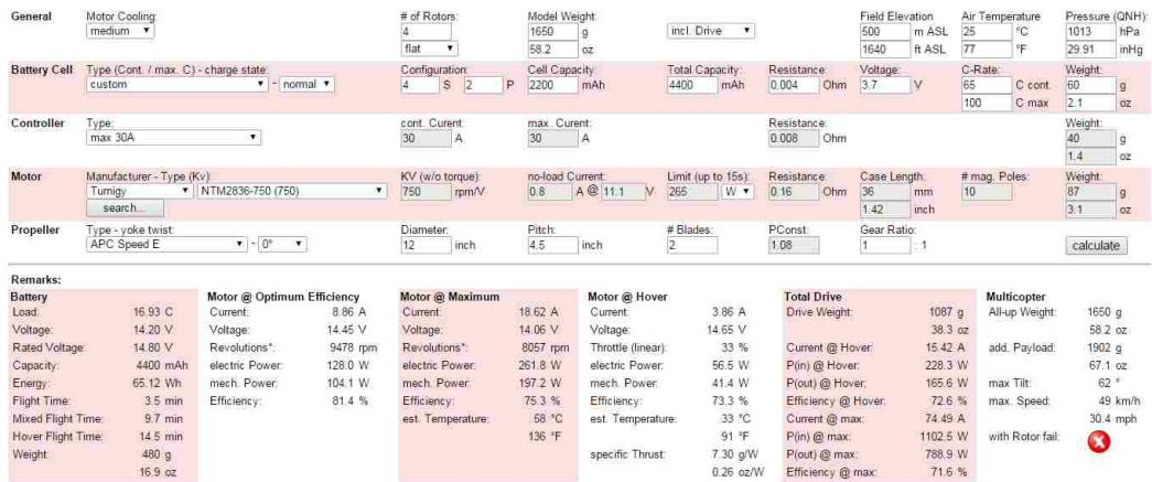
FIGURE 3-7: QUADX PROPULSION AND POWER PERFORMANCE CALCULATION RESULT
