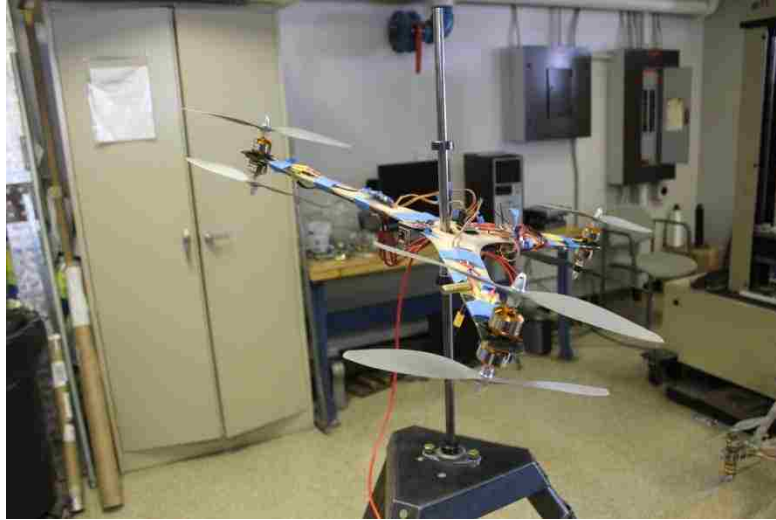
FIGURE 1-5: 2ND GENERATION PROOF-OF-CONCEPT HOPPER SIMULATOR
