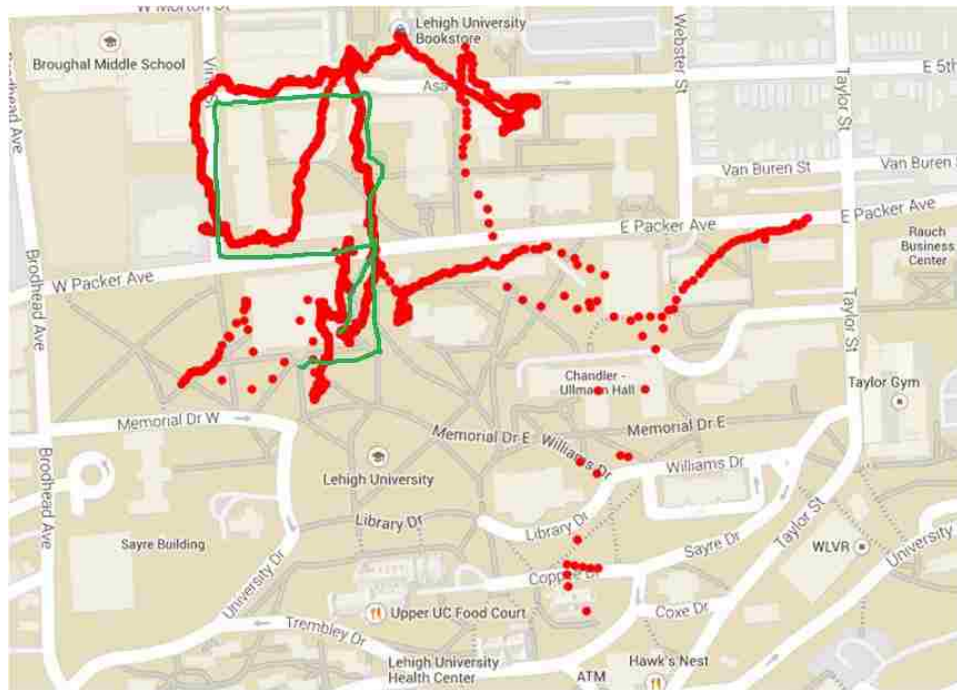
FIGURE 8-4: ACTUAL VS. MEASURED PATH TRAVELLED (GREEN = TRUE PATH / RED = GPS PATH)
