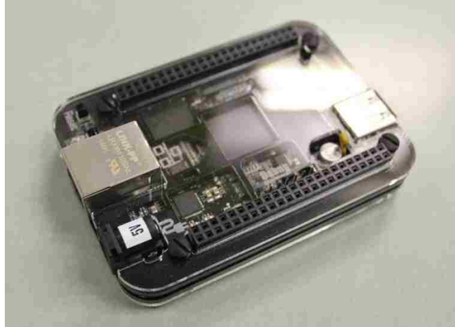
FIGURE 5-6: BEAGLEBONE BLACK IN PROTECTION CASE
