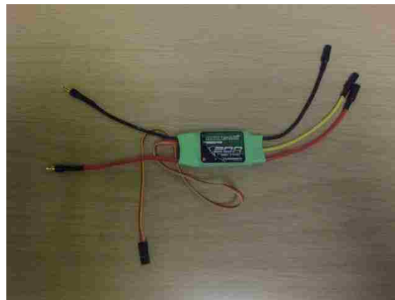
FIGURE 3-5: MULTISTAR 20 AMP 2-4S ESC
