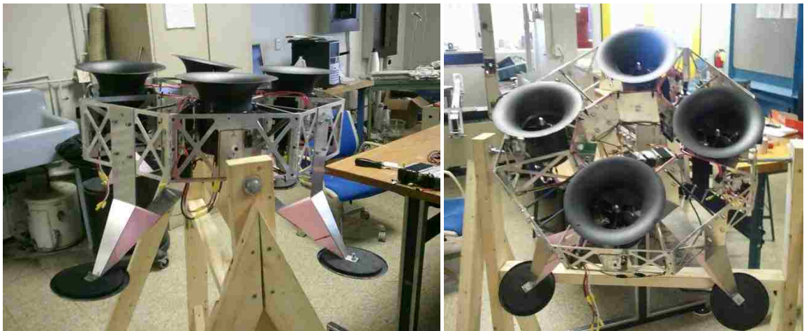
FIGURE 1-3: 1ST GENERATION HOPPER SIMULATOR ON SINGLE-AXIS TEST RIG
