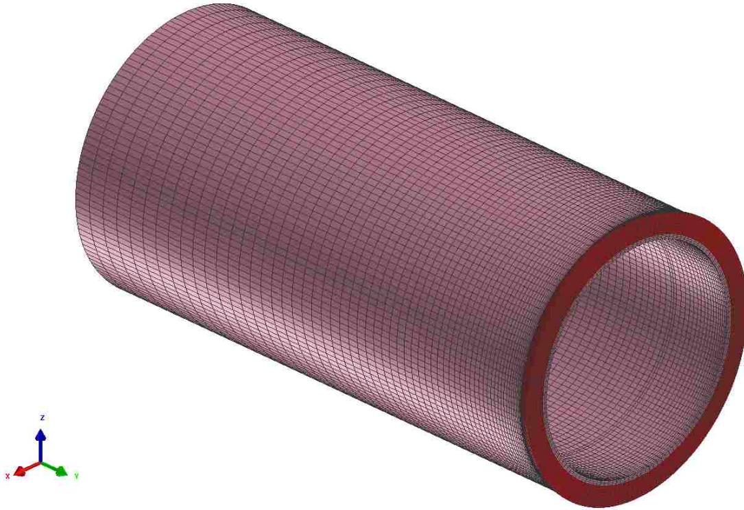
Exhibit 3-1 Half plane 3-D modeling of girth welding of pipe
