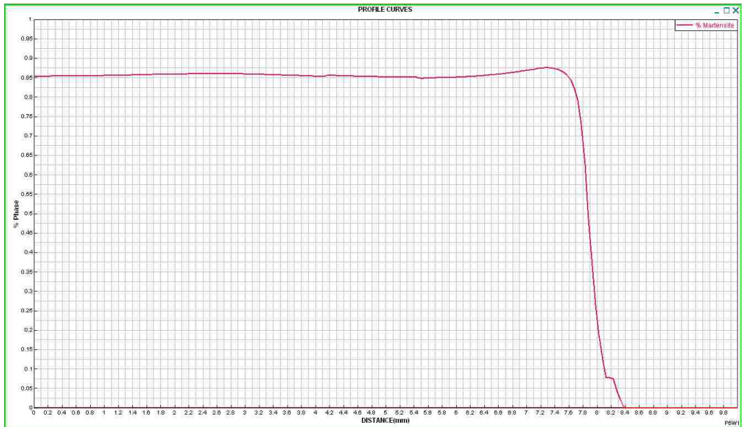
Figure 4.24 Martensite distribution along top surface after cooling
