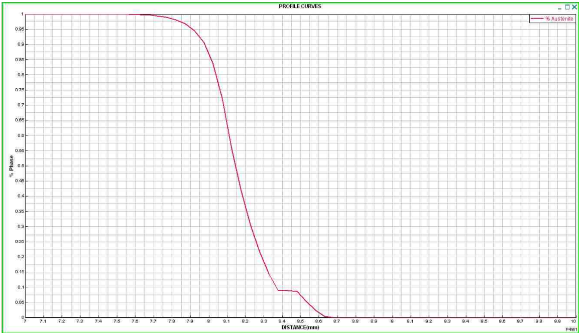
Figure 4.21 Austenite distribution along top surface at 5s during welding
