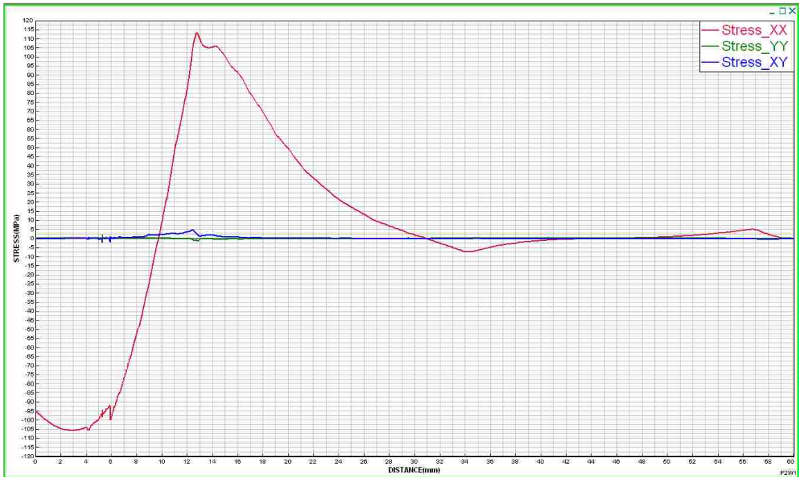
Figure 2.4 Residual stresses on the top surface of flat plate
