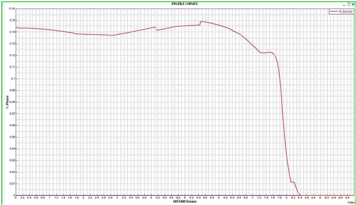
Figure 4.23 Bainite distribution along top surface after cooling
