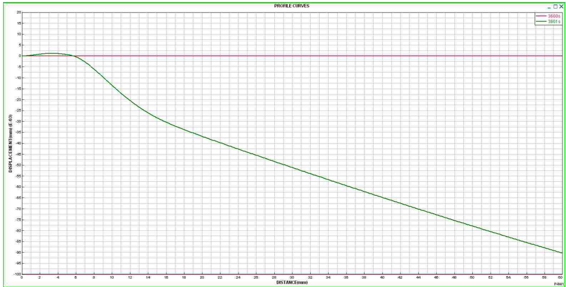
Figure 4.15 Distributions of displacement on bottom-plane for S355J2G3
