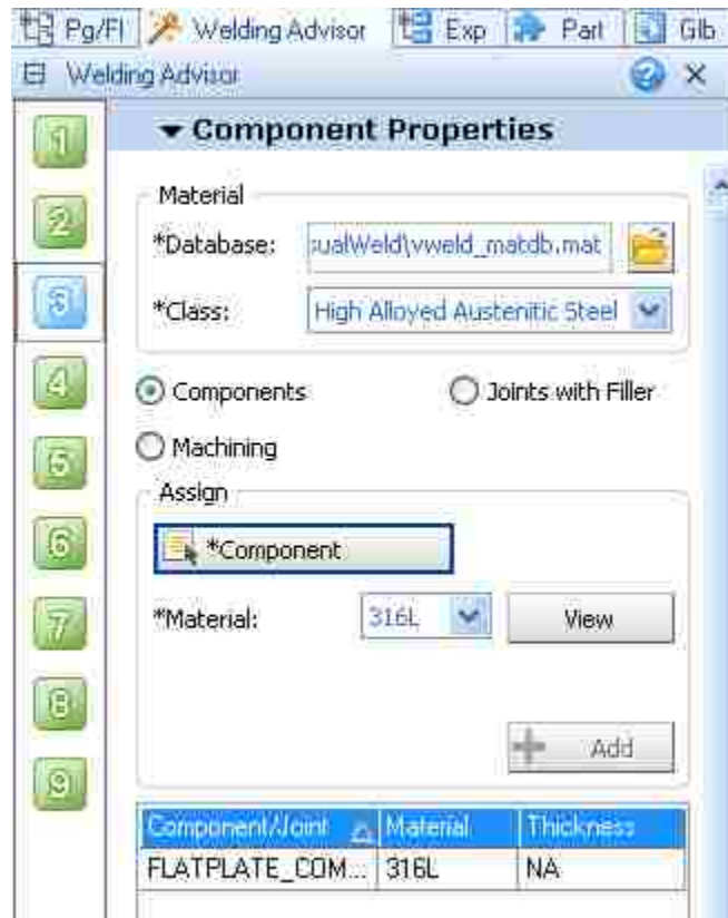
Figure 3.3 Setting up materials of components and joints
