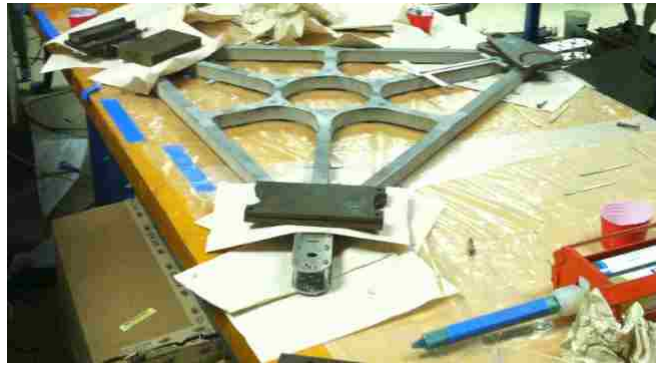
Figure 14: Motor Tab Bonding
