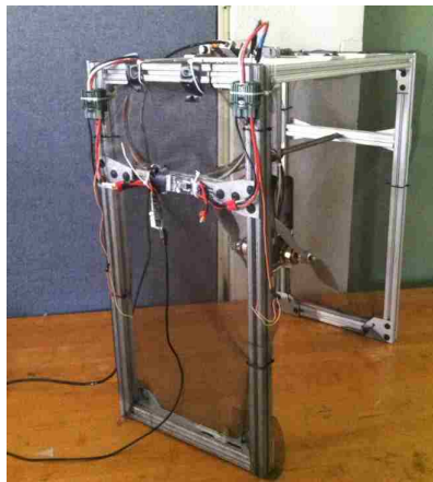
Figure 46: Power Sensors on Thrust Test Stand
