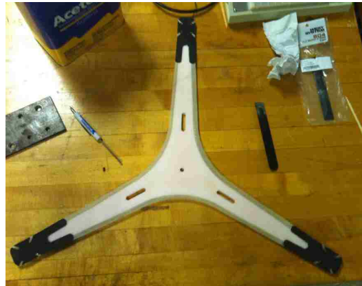
Figure 9: Carbon Stiffeners and Completed Frame
