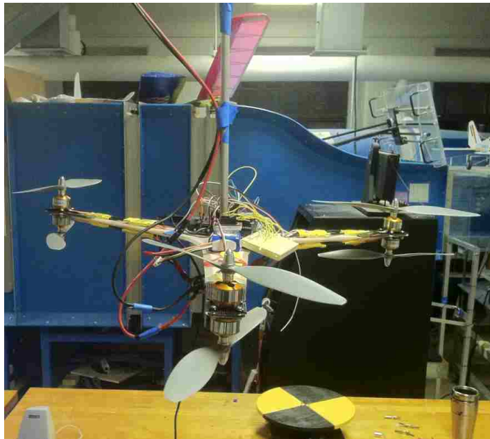
Figure 21: Proof of Concept Vehicle Pole Testing
