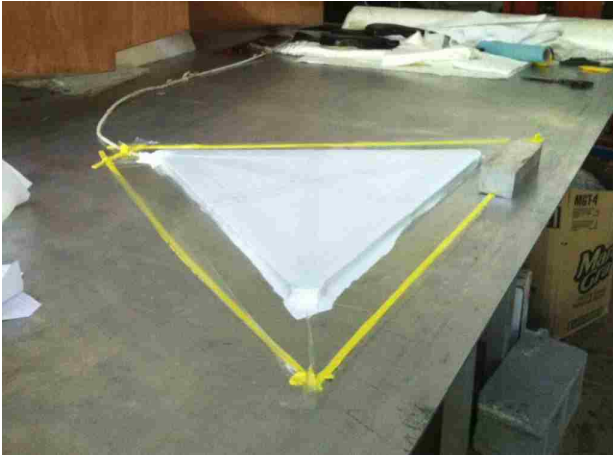
Figure 12: Vacuum Cure of Frame
