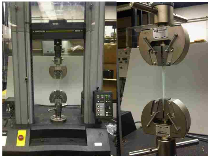
Figure 4.15: INSTRON 5667 C 9620_30 kN Tensile Testing Machine (left) and zoomed in view of a dogbone held in the pliers (right)
