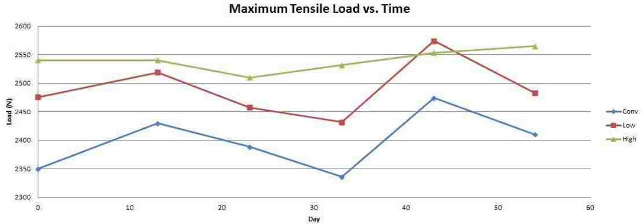
Figure 5.16: Maximum loads vs. incubation time for enzymatic biodegradation
