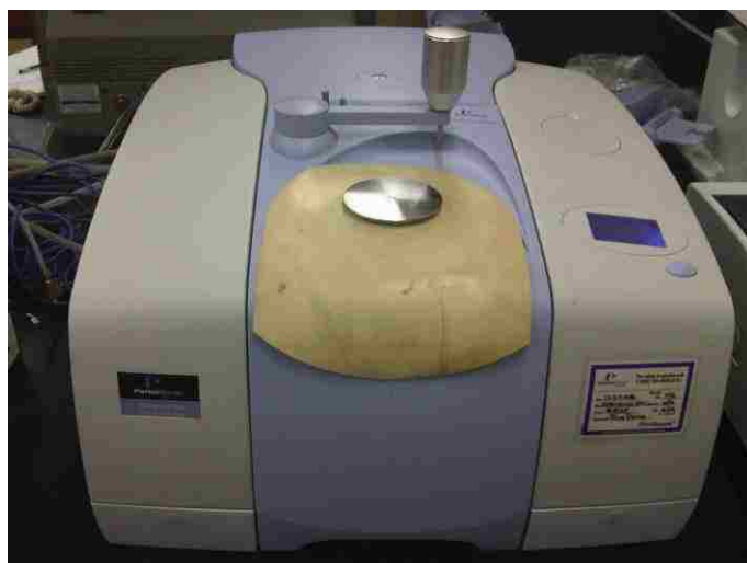
Figure 4.8: PerkinElmer ® Spectrum 100 FT-IR spectrometer
