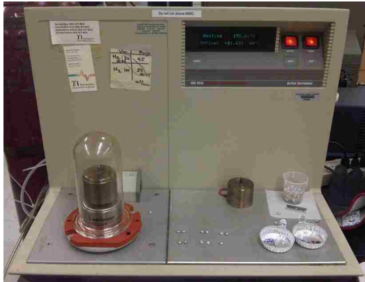
Figure 4.9: DSC 2910 MDSC equipment from Du Pont Instruments™
