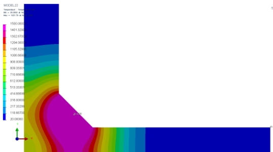
Figure 4.28 Temperature distribution during welding with the finer mesh for 316L (1) at t=1.26s (2) at t=2.52s (3) at t=3.16s
