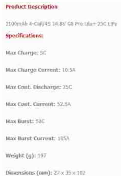
Figure 4-9: LIPO Battery Specifications
