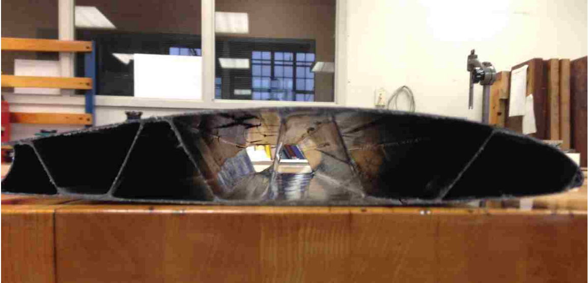
Figure 27: Finished Wing with Internal Structure
