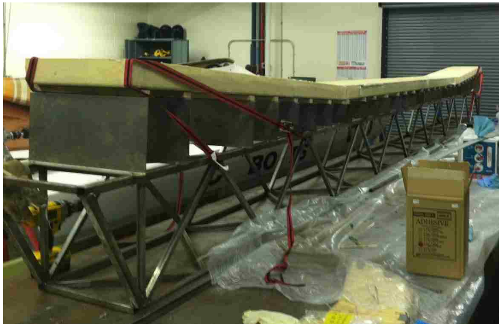
Figure 37: Finished Mold Half
