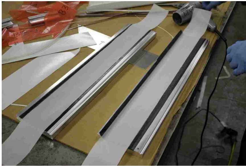
Figure 56: Layup Finished and Ready to Close Molds
