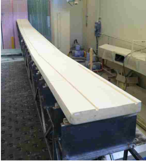
Figure 40: Finished Wing Mold
