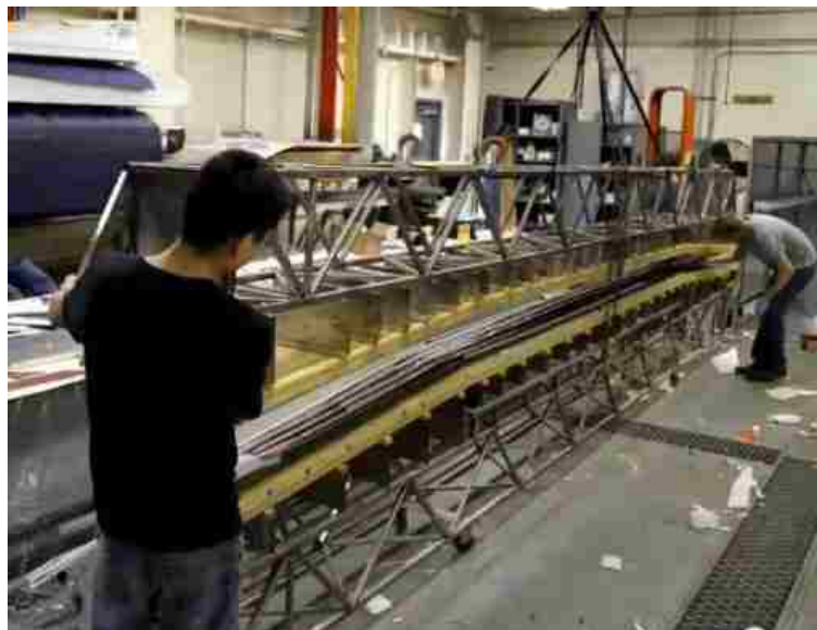
Figure 47: Closing the Wing Mold
