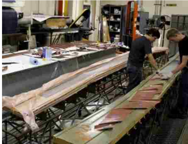
Figure 44: Debulking First Ply and Continuing Layup
