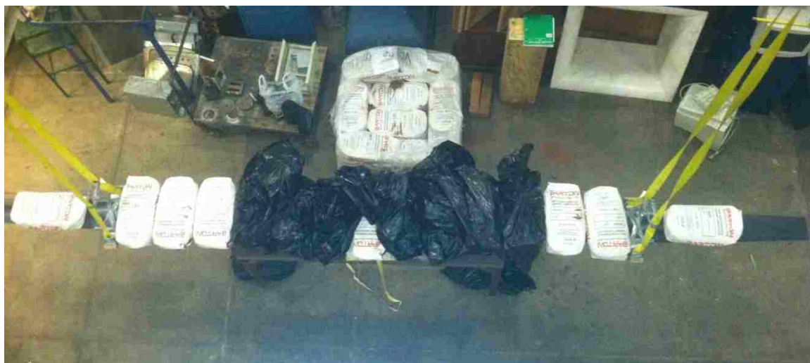
Figure 50: 3.5 KN Proof Load of Wing
