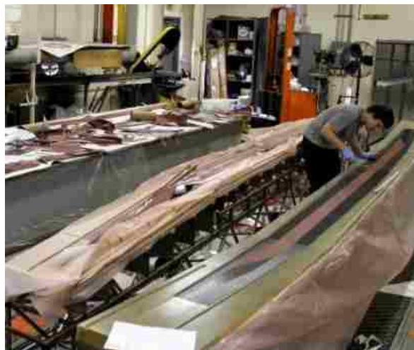
Figure 45: Laying of Wing Spar Plies
