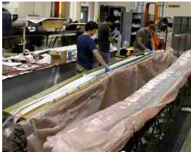
Figure 46: Laying Web Plies over Foam Molds
