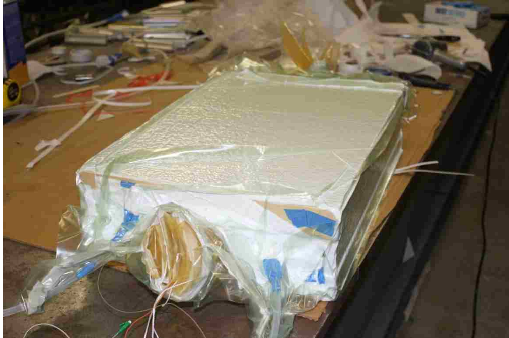
Figure 26: Test Mold Under Vacuum
