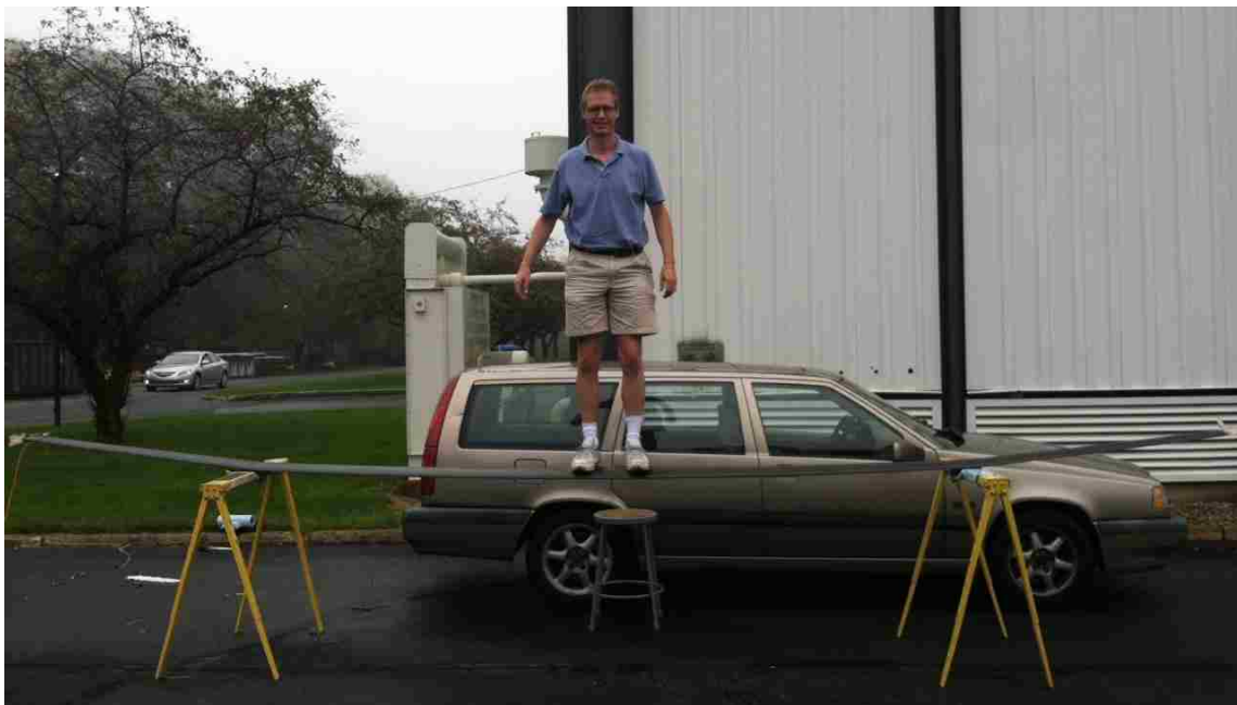
Figure 49: Preliminary Wing Testing
