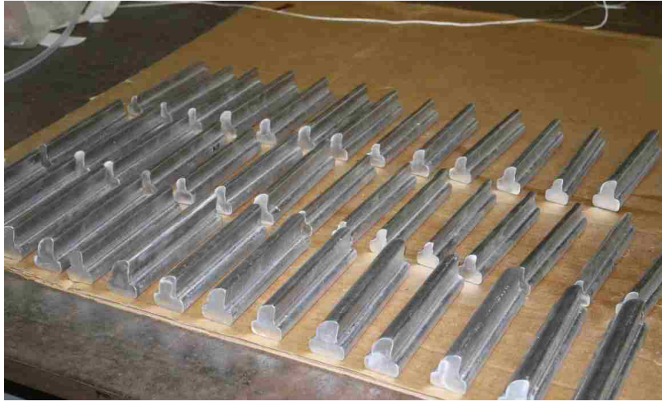
Figure 42: Finished Trailing Edge Inserts
