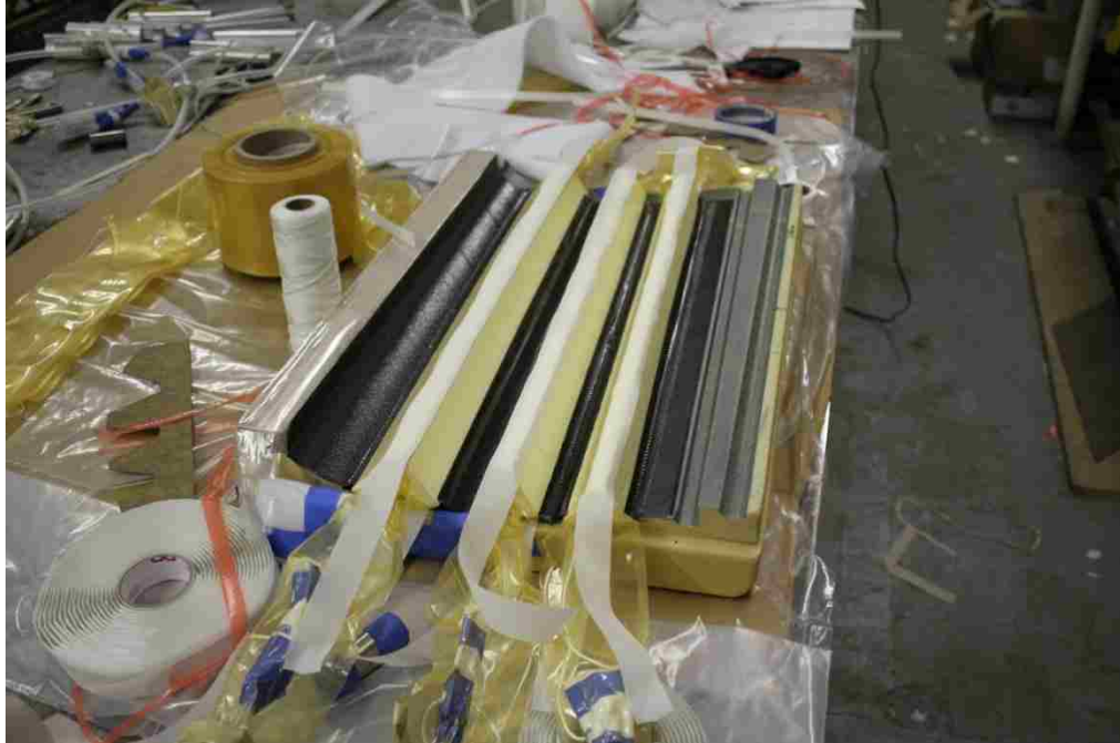
Figure 24: Placement of Foam Molds
