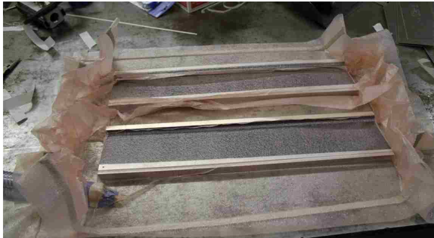
Figure 55: Flap Ply Debulking
