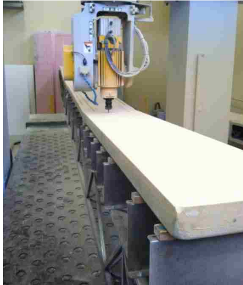
Figure 39: Wing Mold Machining
