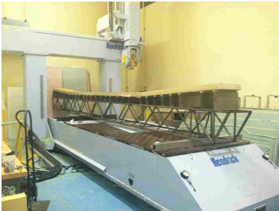
Figure 38: Mold Setup for Machining
