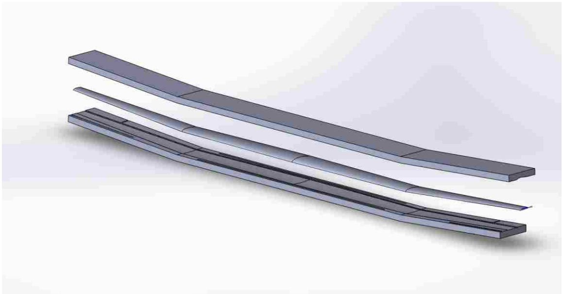
Figure 29: Wing Mold Layout including the Wing (in the center)
