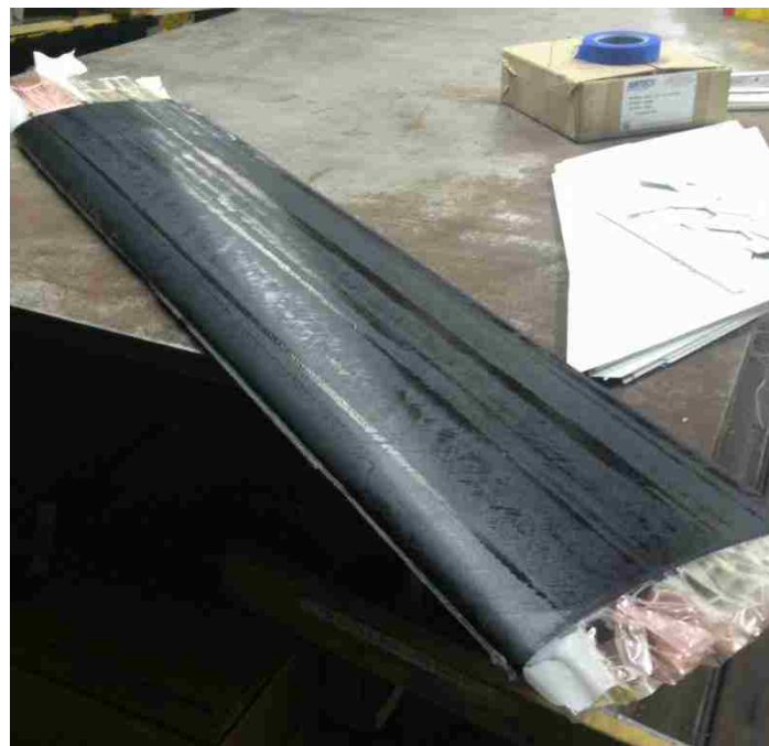
Figure 51: Typical Wing Skin Defects
