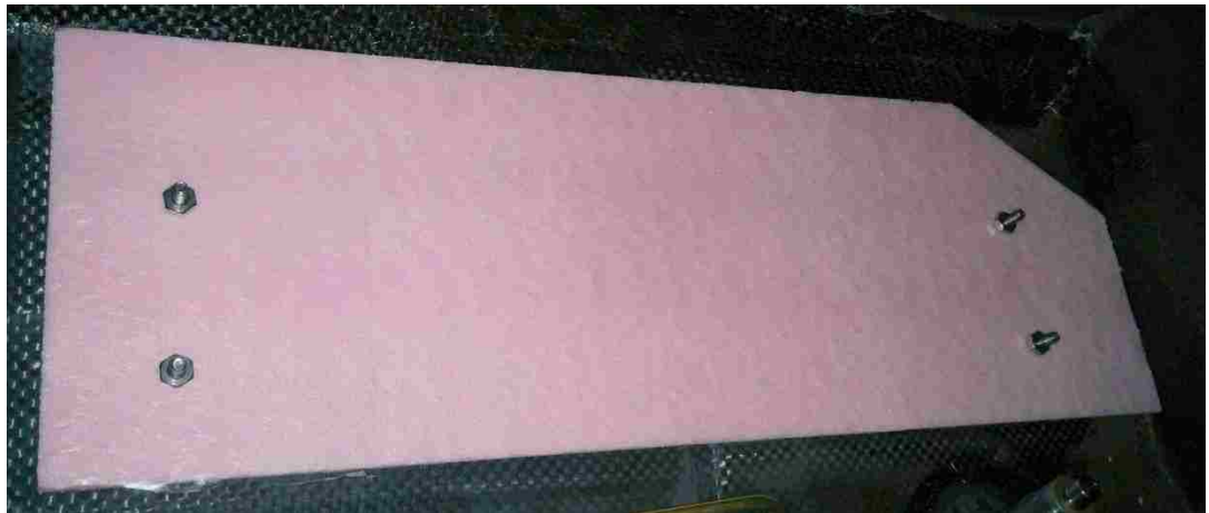
Figure 34: Bonding Mounting Studs for Battery Trays
