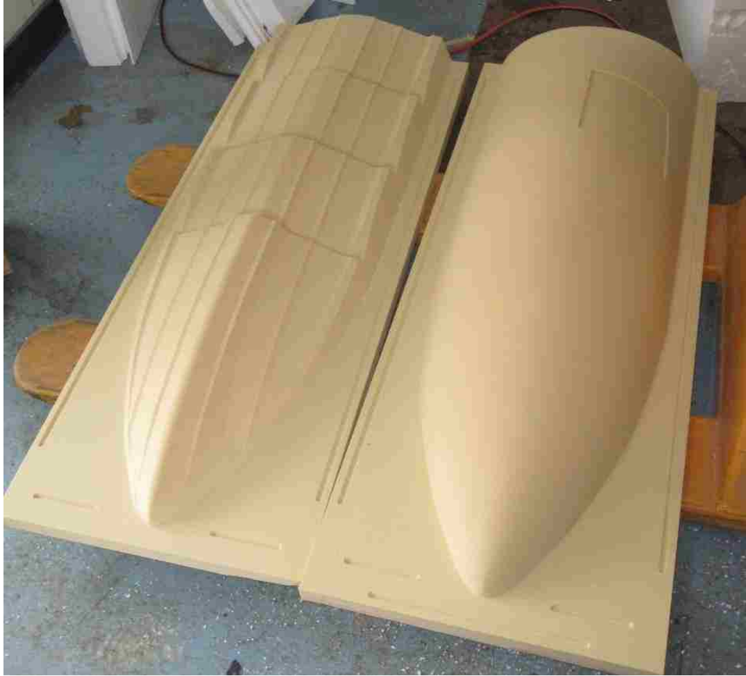
Figure 8: Completed LORCA Mold Plugs
