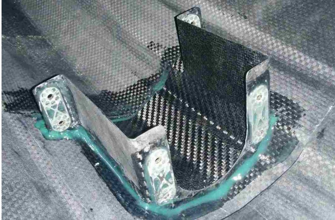
Figure 30: Bonded LORCA Motor Mount
