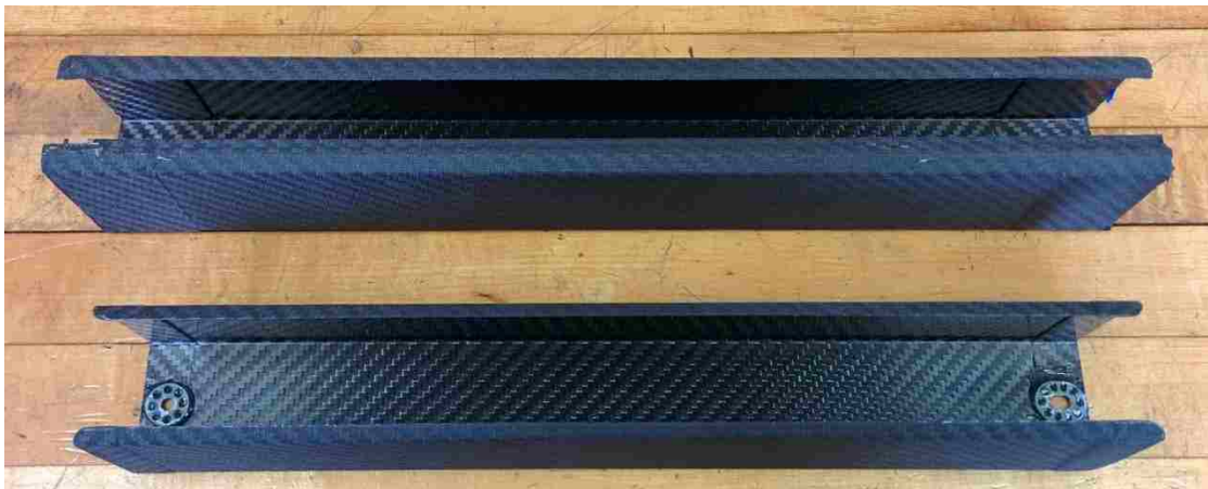
Figure 26: Battery Trays Before and After Trimming
