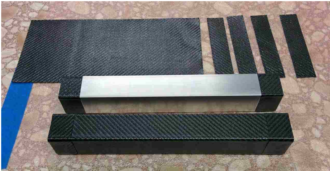
Figure 21: Laying Pre-Preg onto Battery Tray Molds
