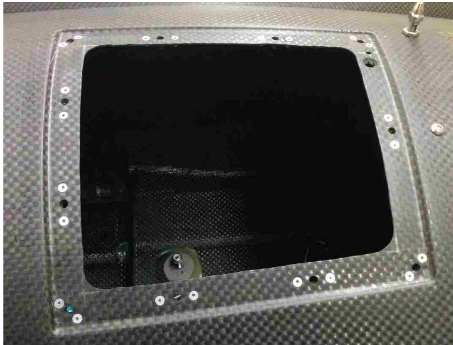
Figure 29: Access Hatch Lip
