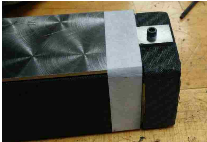
Figure 25: Battery Tray Being Trimmed
