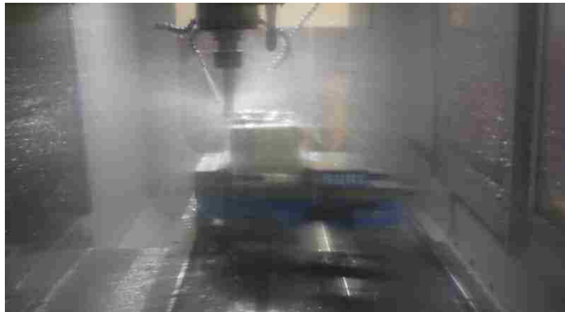
Figure 15: Machining the Motor Mount Mold
