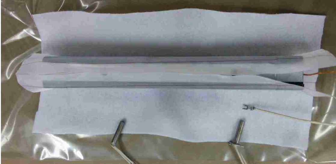
Figure 22: Battery Tray Mold Wrapped with Peel Ply, Breather
