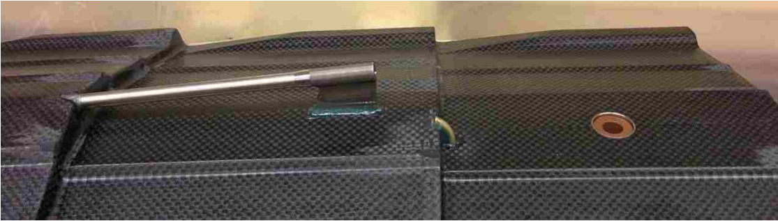
Figure 31: Drive Shaft Supports and Rudder Post Bonded in Place
