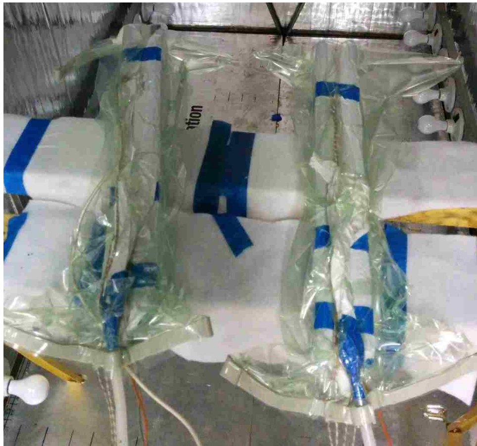
Figure 23: Two Molds Sitting under Vacuum
