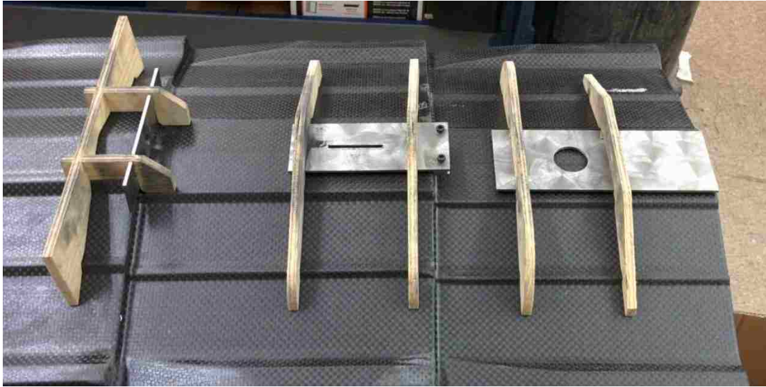
Figure 27: Hole Patterns on a LORCA Hull
