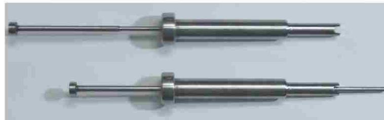
Figure 2-10 Actual valve stem with ejector pin [2]
