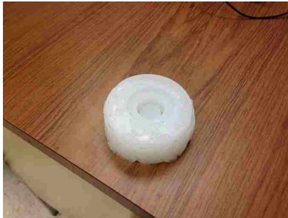
Figure 17: Membrane mold made by the silicon rubber
