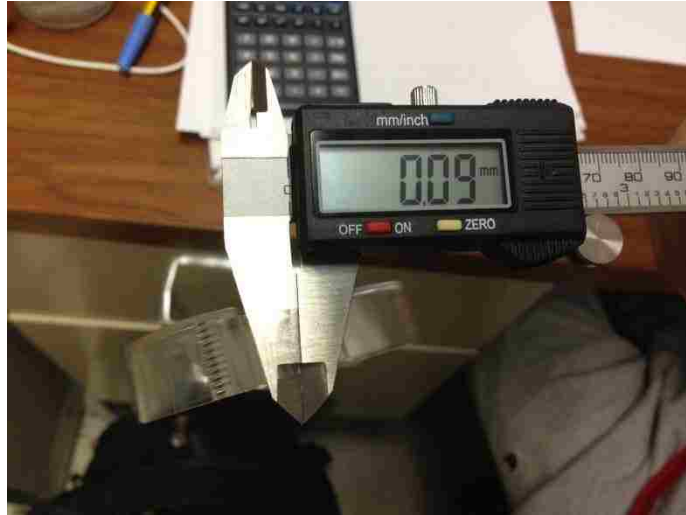
Figure 32: Thickness of the plastic tape
