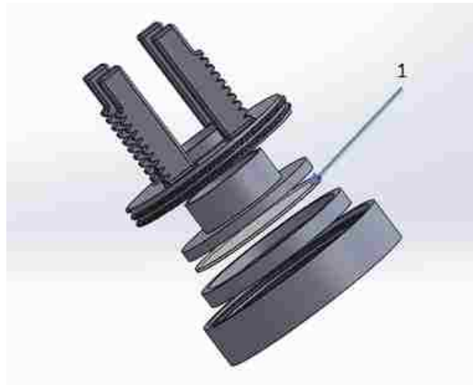
Figure 39: Assembly of all parts for the working component: 1.Membrane
