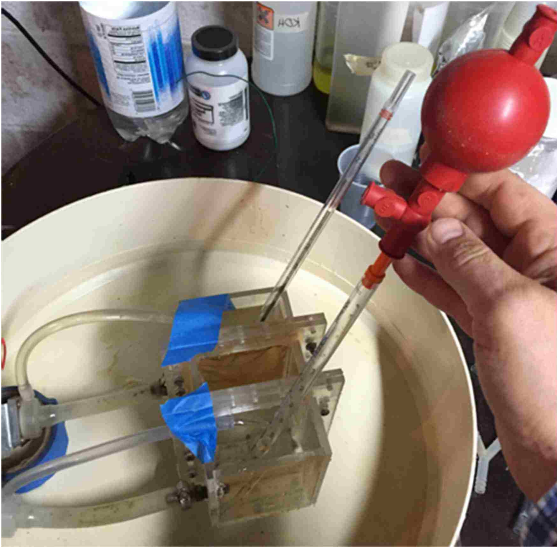
Figure 21. Experimental set up for ion exchange membrane experiments
