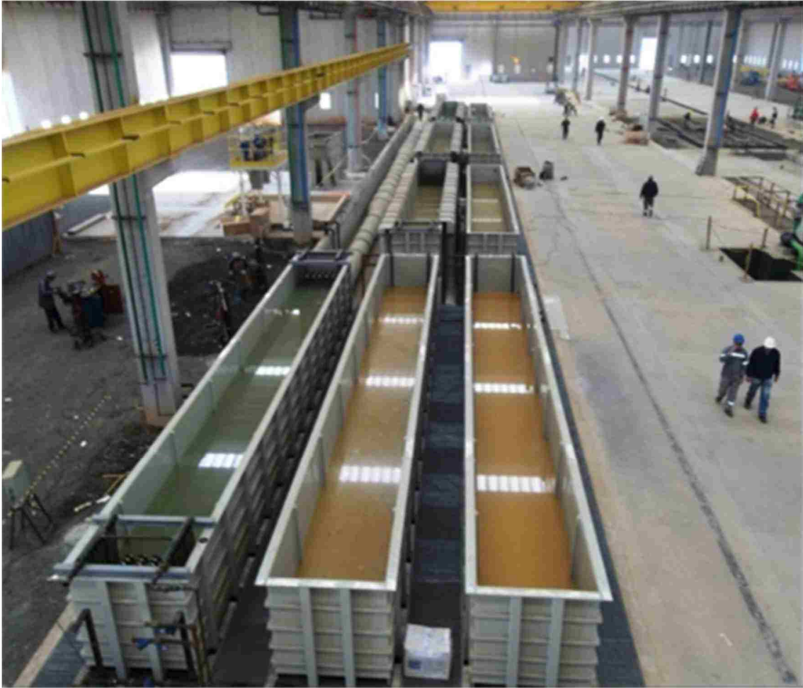
Figure 2. Example of steel pickling process (Covino Jr, 1987)
