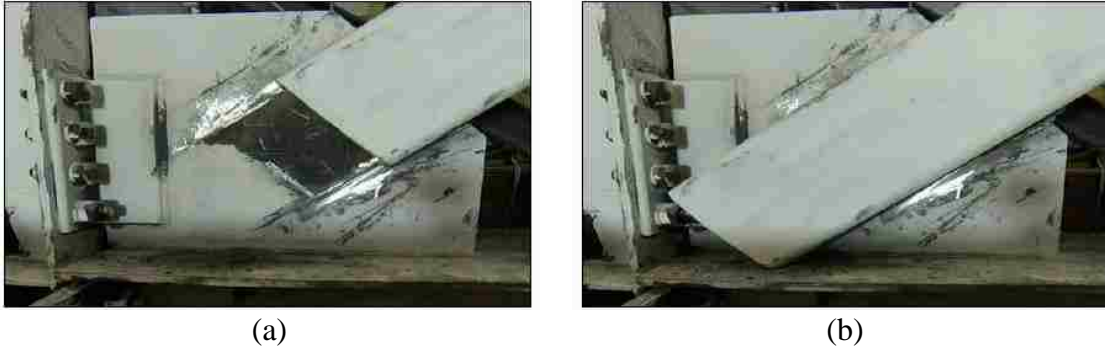
Figure 2.4 (a) brace-gusset weld fracture; (b) brace re-engagement (Sizemore et al. 2015)
