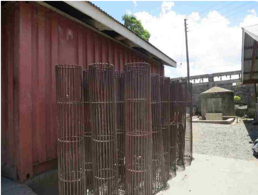
Figure 11.4. Steel tubes used for spacing the bones inside the furnace for more uniform air flow.
