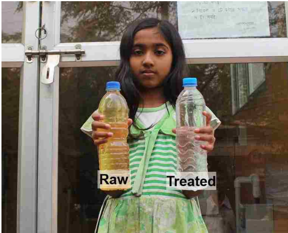
Figure 7.13. A community member holding a bottle of raw groundwater and a bottle of HAIX-NanoZr treated water. Notice the aesthetic difference in water quality due to concurrent iron removal: 4.3 mg/L \rightarrow <0.1 mg/L.
