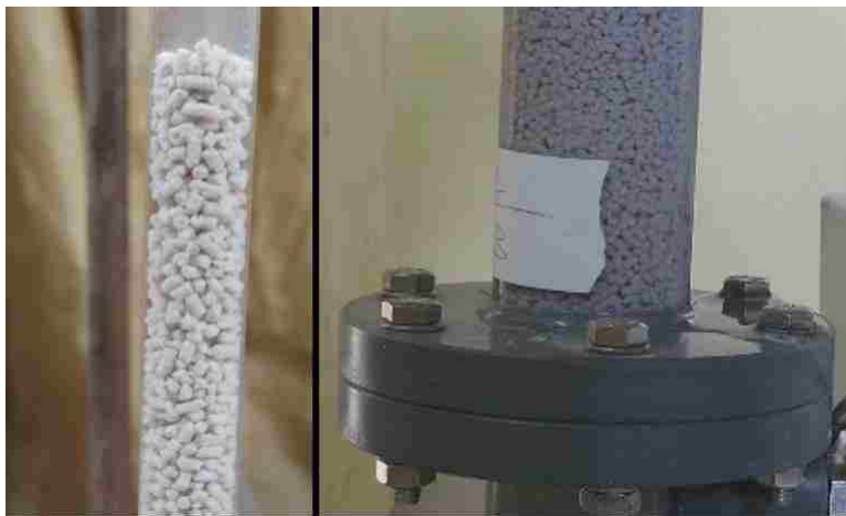
Figure 3.7. Poor hydraulics with testing HAP in ACE Glass columns from Lehigh (L). Plug flow with HAP in wider diameter column (R).
