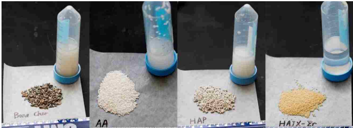
Figure 4.10. Fluoride adsorbents after a 12 hr shake test: bone char (BC), activated alumina (AA), hydroxyapatite (HAP), and HAIX-nanoZr (from left-right). Images by Jinze Li.
