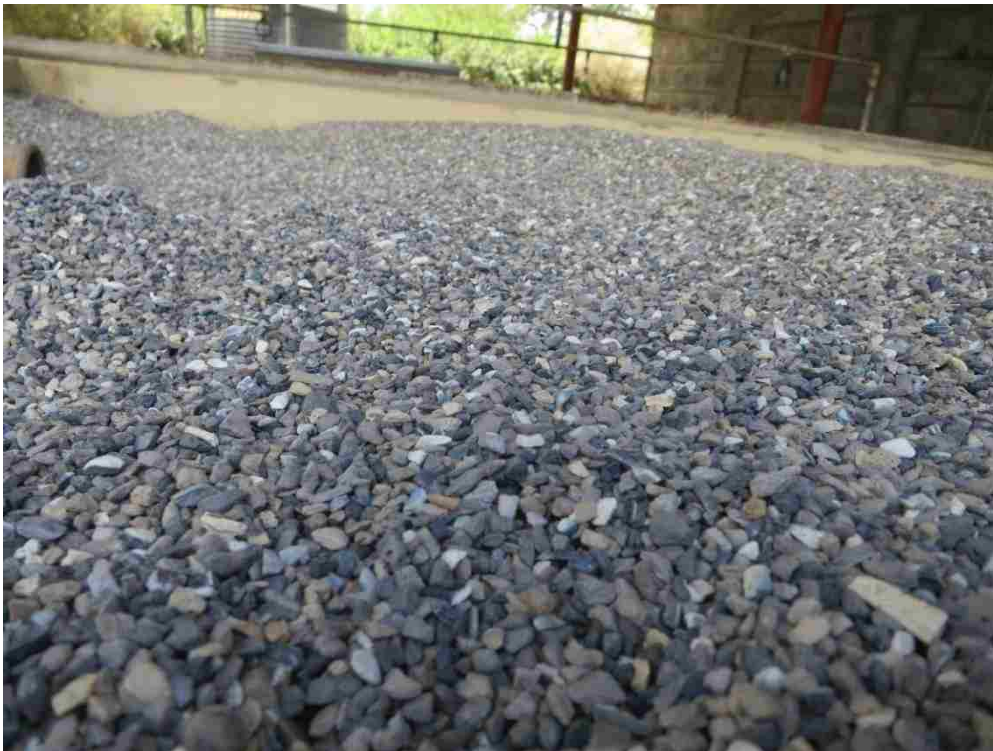
Figure 11.5. Charred bone pieces in the washing tank where charred-on organics are removed with a dilute acid wash.
