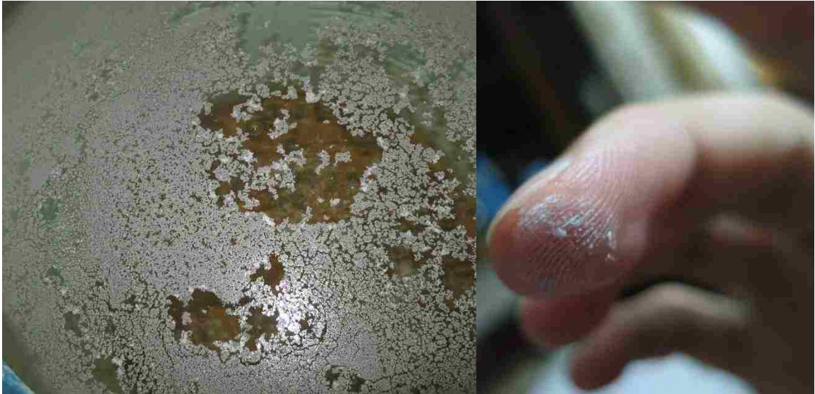
Figure 2.15. Calcium carbonate precipitation present in the A) treated effluent from the arsenic treatment system on May 14, 2013 (L) and B) calcium carbonate from the side of the treated water tank.
