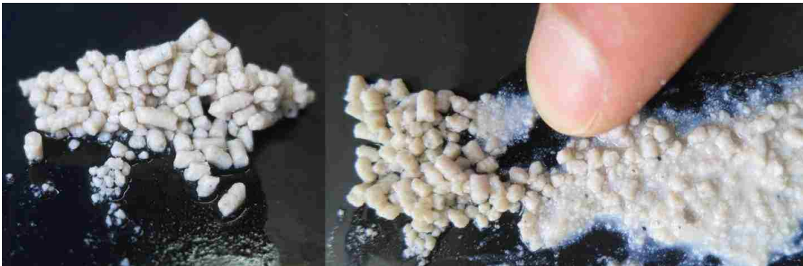
Figure 4.3. Wet HAP on a table (L); the same wet HAP moments later after light pressure (R).
