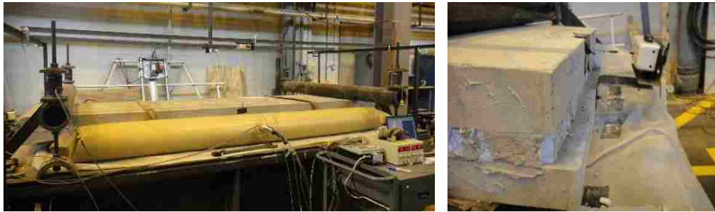
Figure 37: Center-span displacement and end-slip instrumentation
