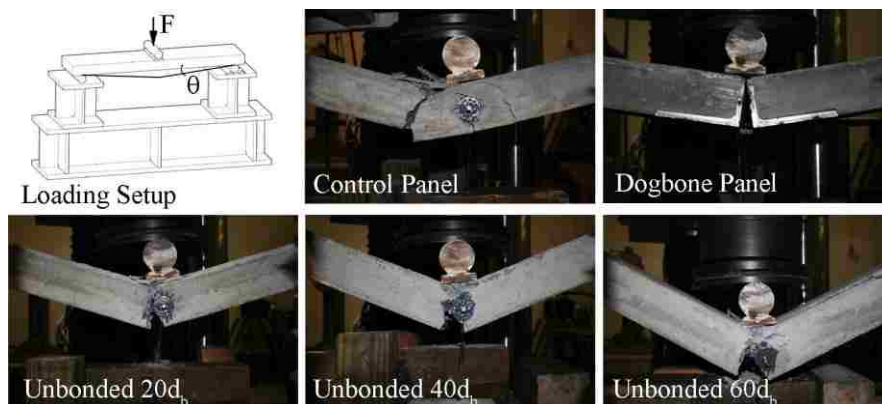
Figure 23: Loading setup and panels at ultimate
