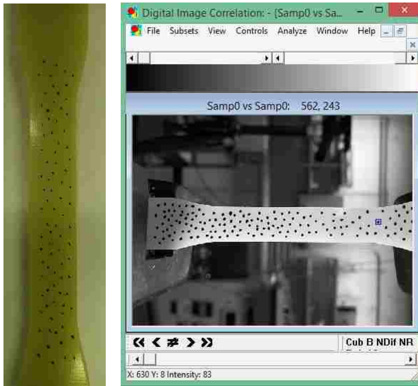
Figure 57: Typical speckle pattern and digital image correlation
