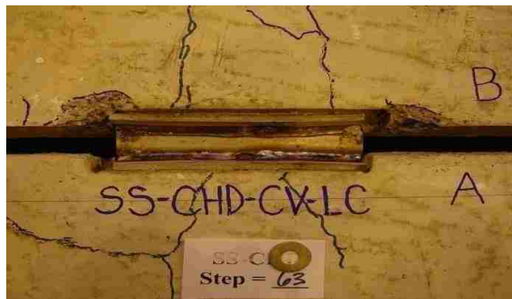
Figure 4.41. Damage state at 0.80-in shear opening
