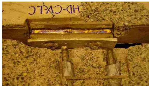
Figure 4.42. Damage state at 1.60-in shear opening
