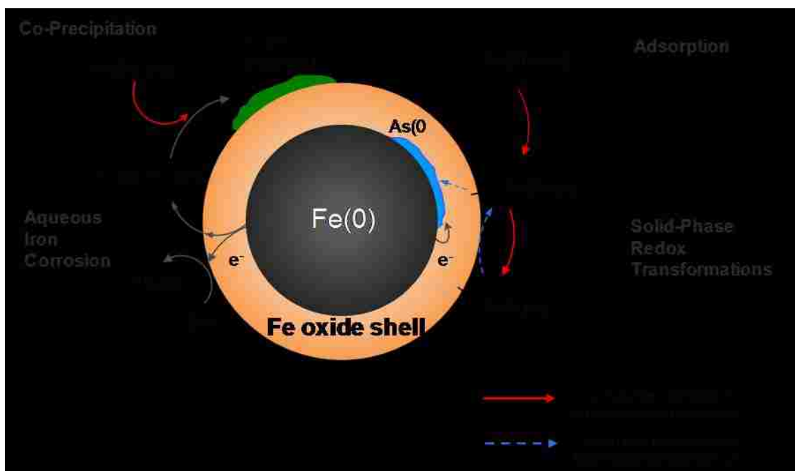
Figure 7.17 Schematic diagram summarizing processes responsible for arsenic removal in As(III)-nZVI system in anoxic conditions. The relative scale of the core and shell components of nZVI are for illustration only and do not reflect actual dimensions. As(III) may be taken up from the aqueous phase by adsorption or co-precipitation. The solid-bound As(III) is oxidized rapidly at the oxide surface, and the As(V) formed may be reverted to As(III) at a slower rate. Some As(III) diffuses towards Fe(0) core and is reduced to elemental arsenic (As(0)) near the oxide/Fe(0) interface.
