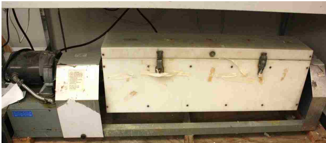
Figure 2.1 Rotary shaker for material preparation and batch test
