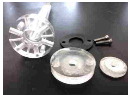
Figure 2.3 Schematic of the batch kinetic test apparatus and stirrer assembly
