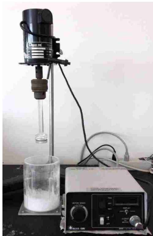
Figure 2.3 Schematic of the batch kinetic test apparatus and stirrer assembly
