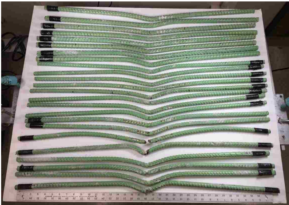
Figure 49: Comparison of Test Specimen Connector Bar Damage
