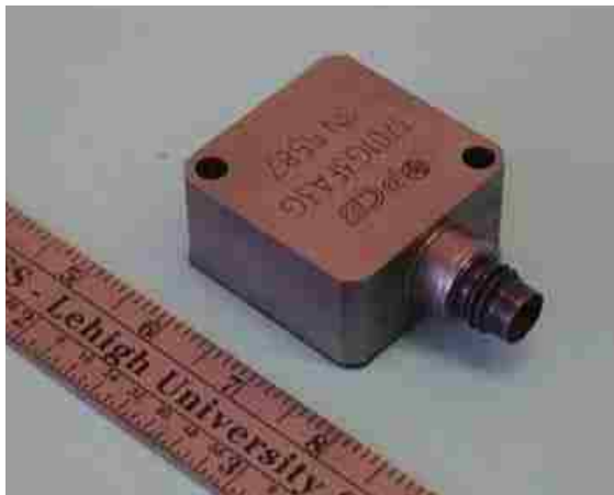
Figure 2.2 PCB wired sensor (courtesy of Mr. Ian C. Hodgson)
