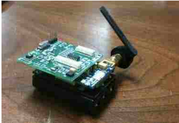
Figure 2.1 'Stacked' wireless sensor node
