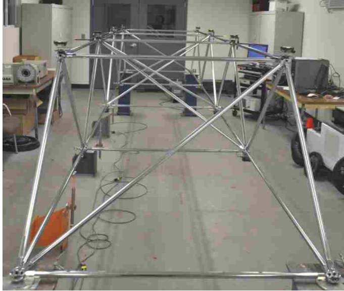
Figure 2.7 3D steel truss of the experiment
