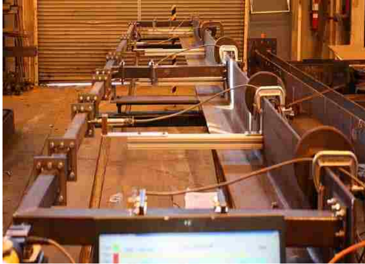
Figure 5.4 The two-bay steel frame
