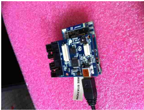
Figure 2.4 Base-station of wireless sensor network: an interface board is stacked on top of an Imote2
