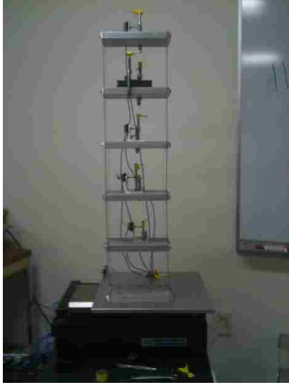
Figure 10.7 The 5 DOF plexiglass-aluminum model
