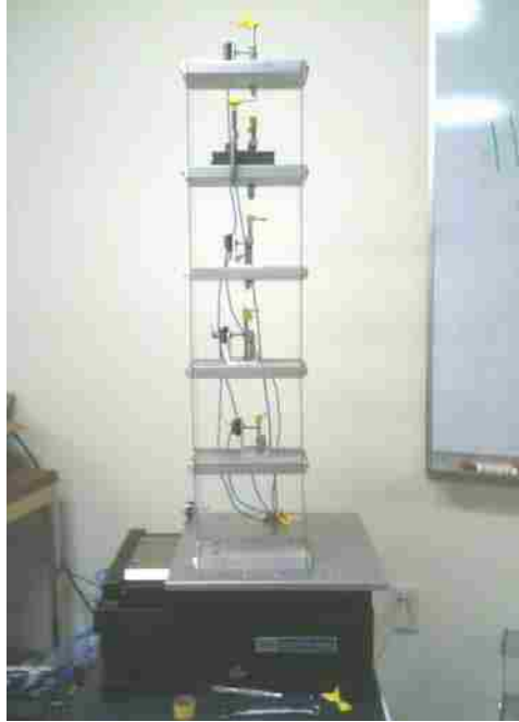
Figure 3.5 The Plexiglass 5-dof lab specimen
