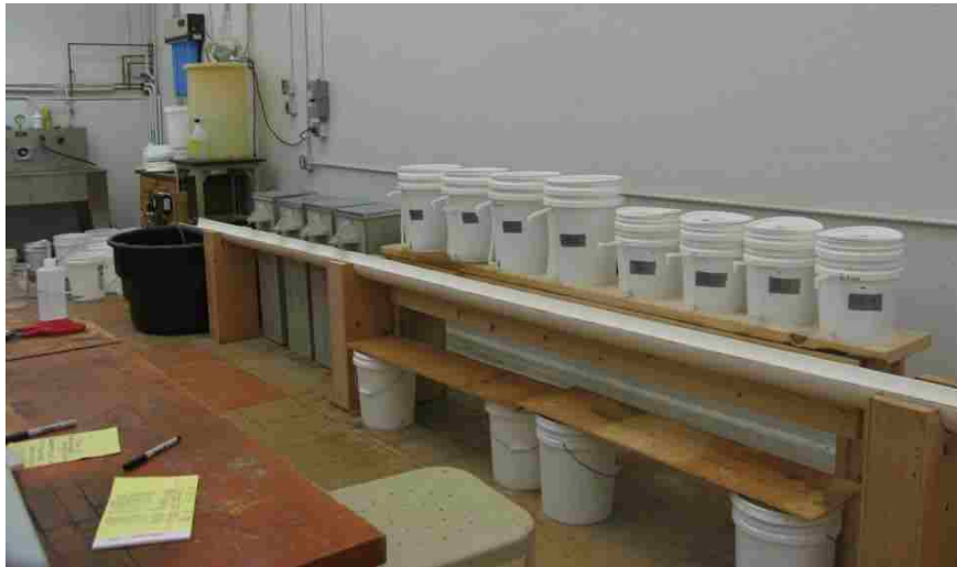
Figure 3. Photograph of laboratory setup. The four concrete BSFs located on the left, the four 5-gallon bucket BSFs are located in the center, and the four 2-gallon bucket BSFs are located on the right. Photo Credit: J. Napotnik
