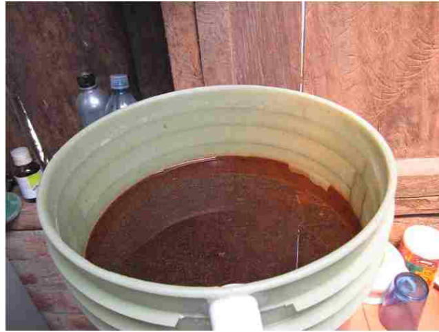
Figure 51. Photo of characteristic contaminant deposition observed in the 5-gal bucket BSF communities. Photo credit: J. Napotnik
