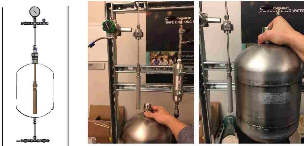
Figure 3-4. carbon dioxide diffuser system for the regeneration tank.
