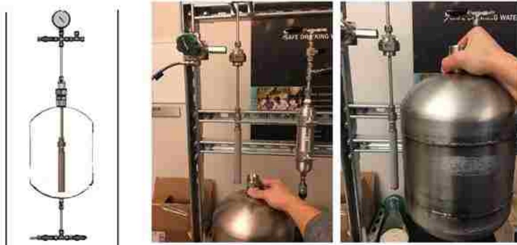
Figure 3-4. A diffuser (left) placed within the regeneration tank to sparge carbon dioxide efficiently in water as the regenerant solution. 18
