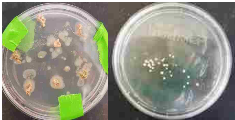
Figure 5-4. Agar-loaded petri dishes to show bacterial presence on the MetaMateria (left) and ion exchangers (right) after 24 hours.
