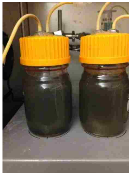
Figure 2.2 The sketch map and pictures of anaerobic test reactors and its water displacement instrument.
