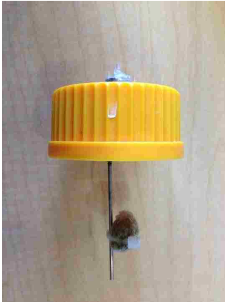
Figure 2.3 The configuration of ion exchange fiber hung in the tube.
