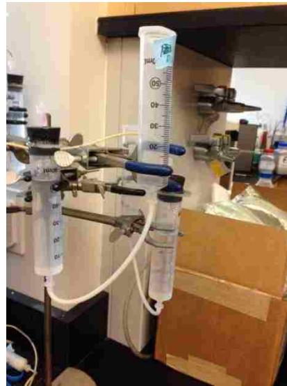
Figure 2.2 The sketch map and pictures of anaerobic test reactors and its water displacement instrument.
