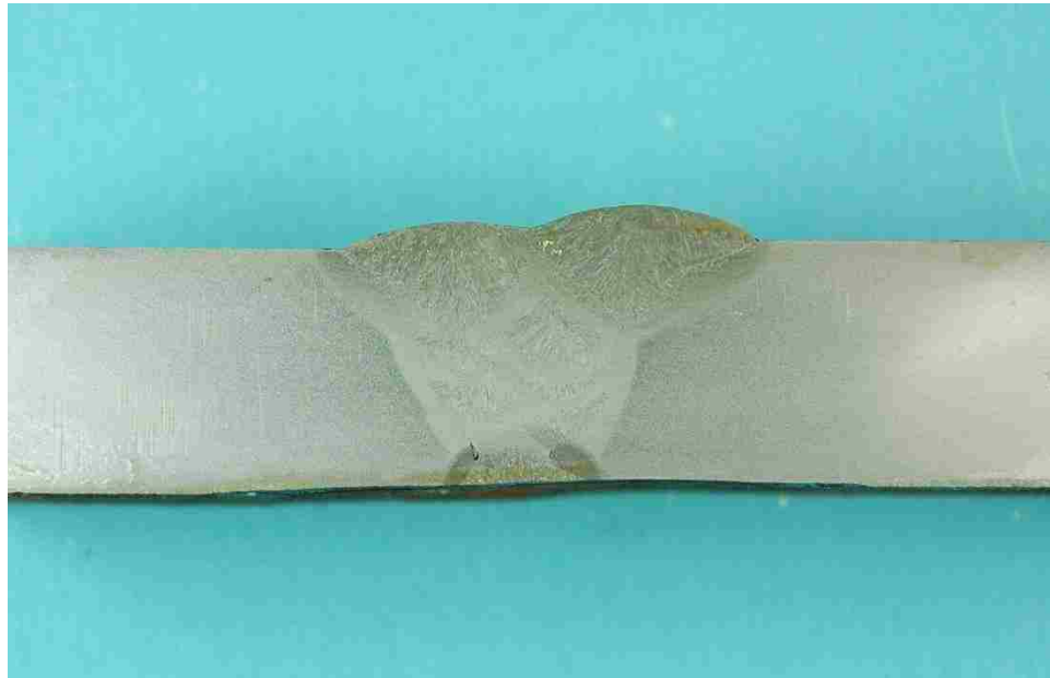
Figure 164 Macro-etched section 3 of CJP deck weld
