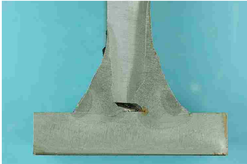
Figure 150 Macro-etched section FS_N_C
