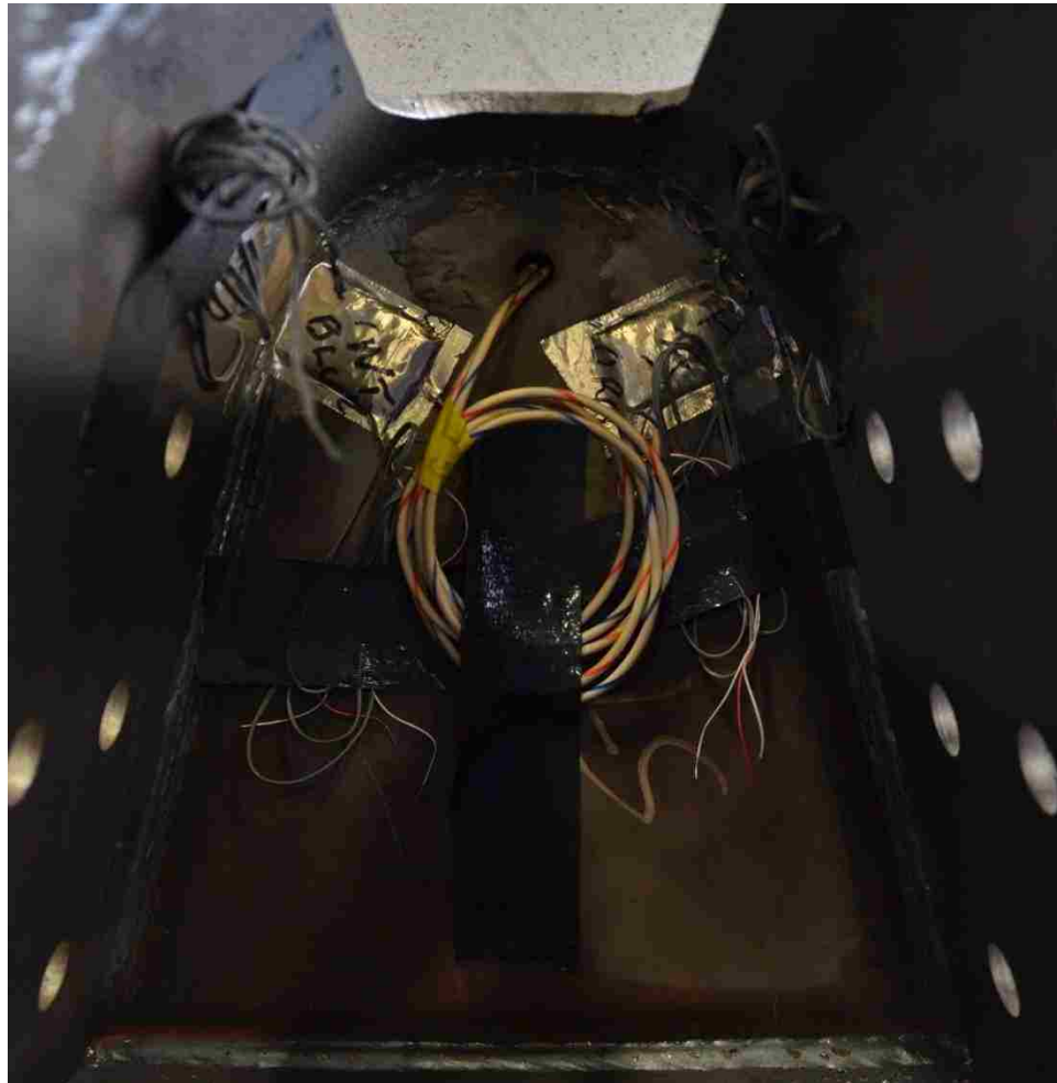
Figure 128 Installation of gauges on rib wall and sealing plate at rib-to-sealing plate connection at HIS facility
