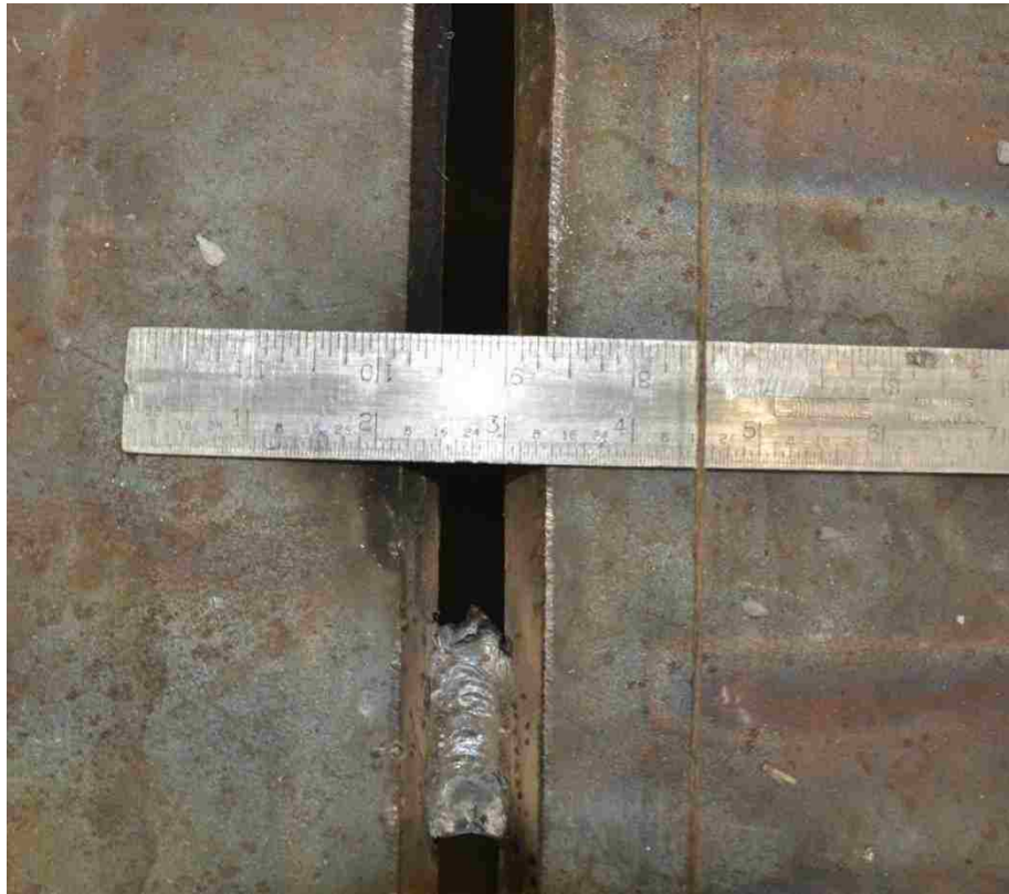
Figure 111 Maximum root gap of 1/2 in.
