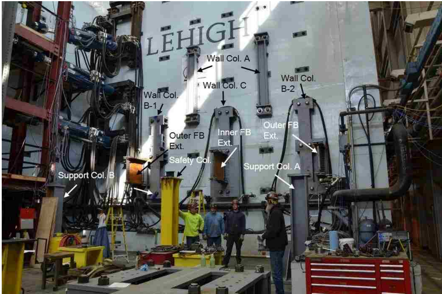
Figure 103 Fixtures for the prototype deck
