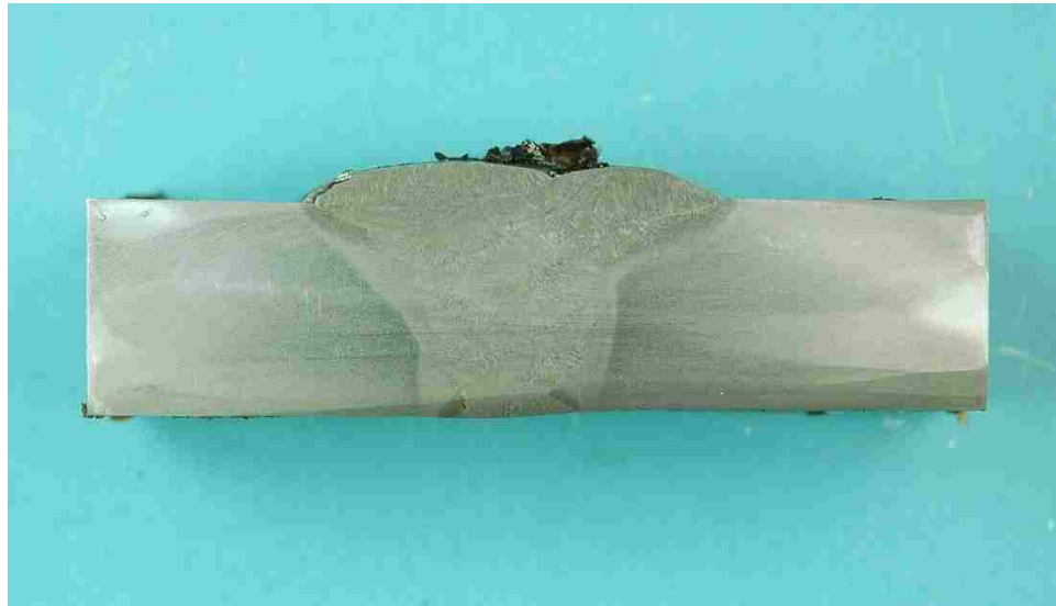
Figure 168 Macro-etched section 5 of CJP deck weld
