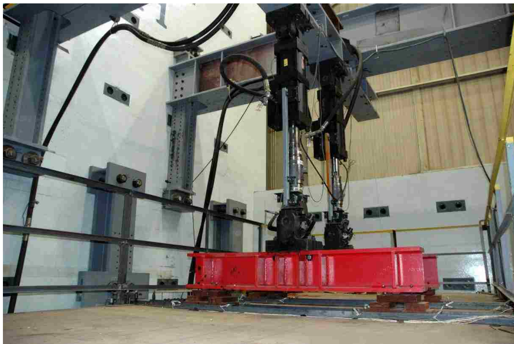
Figure 140 Arrangement of above-deck actuators
