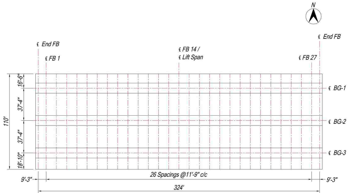
Figure 2 Framing plan of the bridge deck
