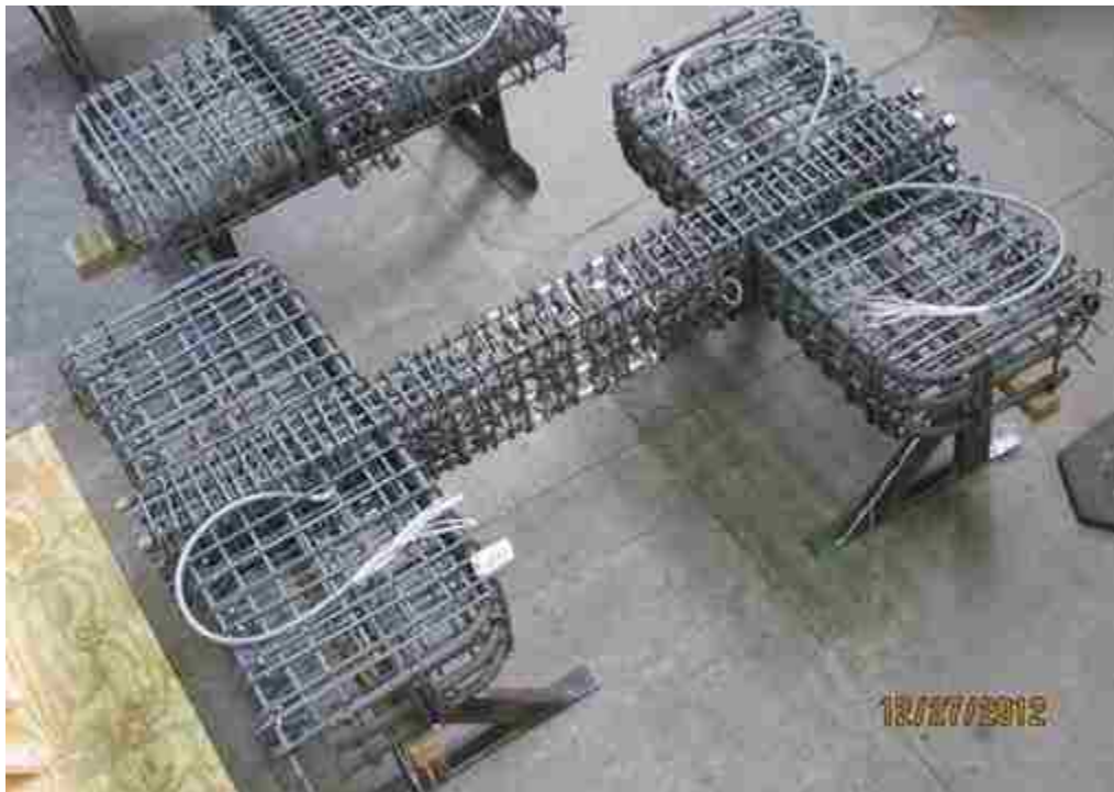
Figure 3-36: Reinforcement of TS02
