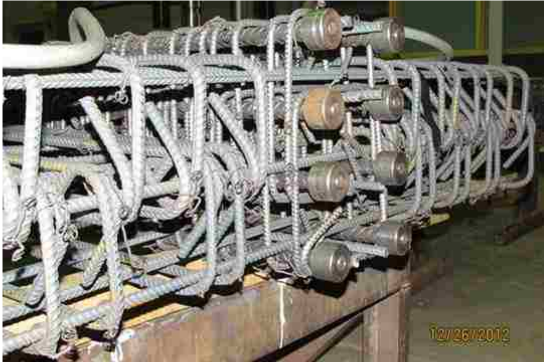
Figure 3-39: Headed bars used in confined concrete column
