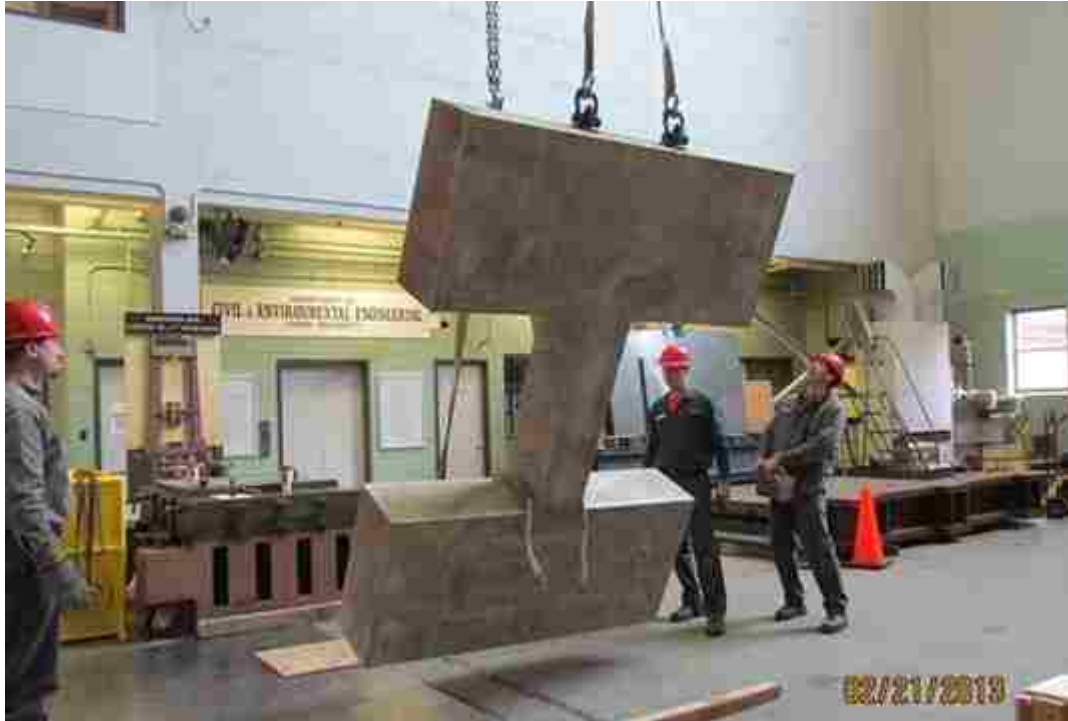
Figure 3-48: Transferring test specimens using a crane
