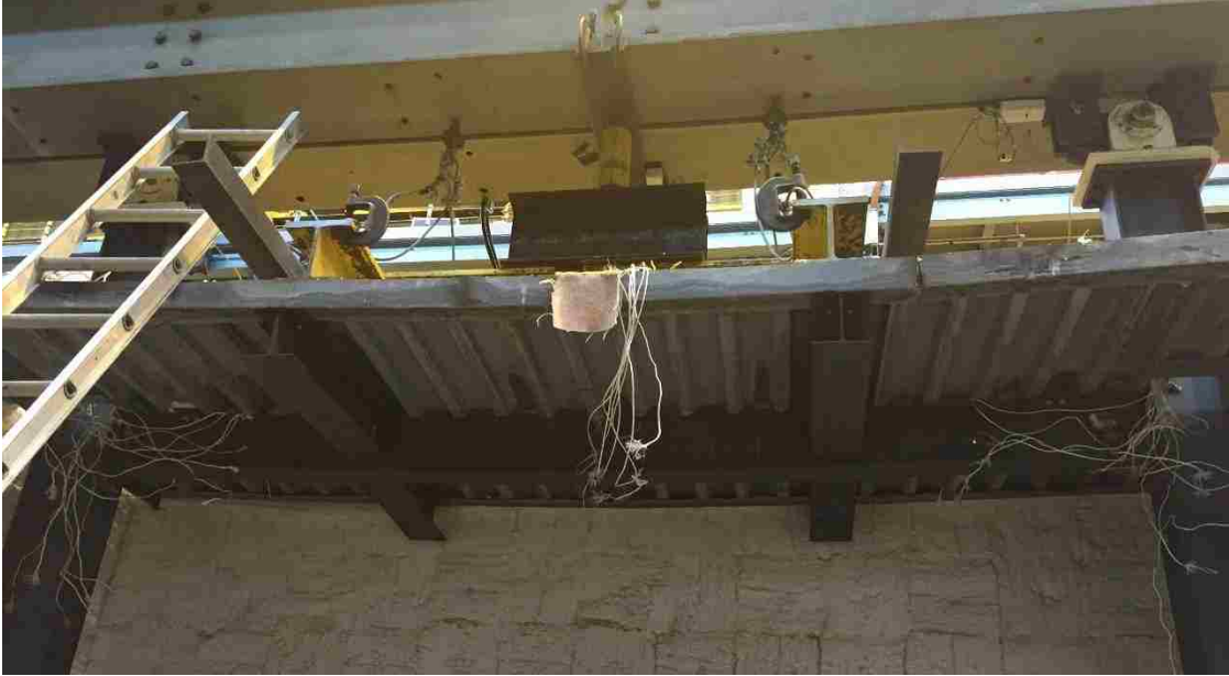
Figure 12 – W8x10 after the test
