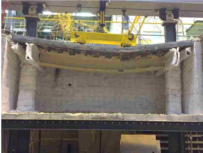
Figure 50 – Protected Beam after Failure
