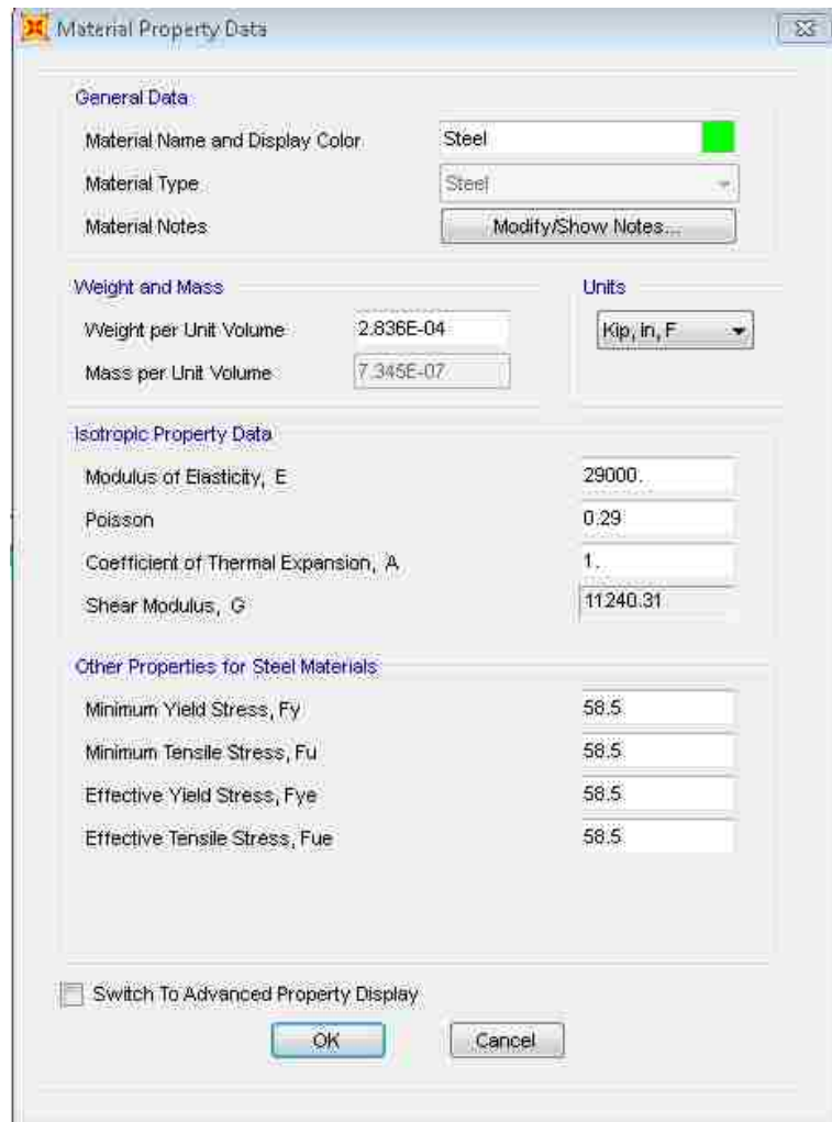
Figure 4.2.1.1: Example of Material Definition Window for SAP2000
