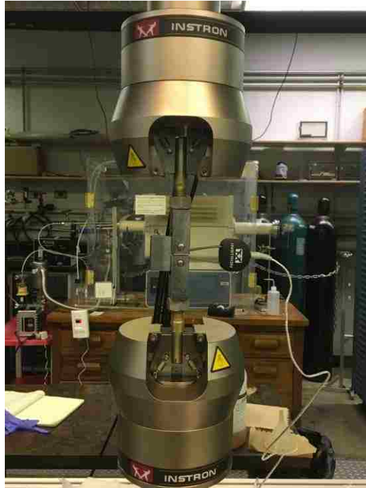
Figure 55 – Compact tension fracture toughness test showing COD clip gauge.
