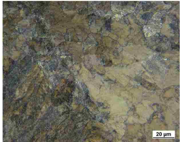
Figure 24 – LOM photomicrographs of Sample 4 from HAY84 rail as viewed at the mid length of the sample.
