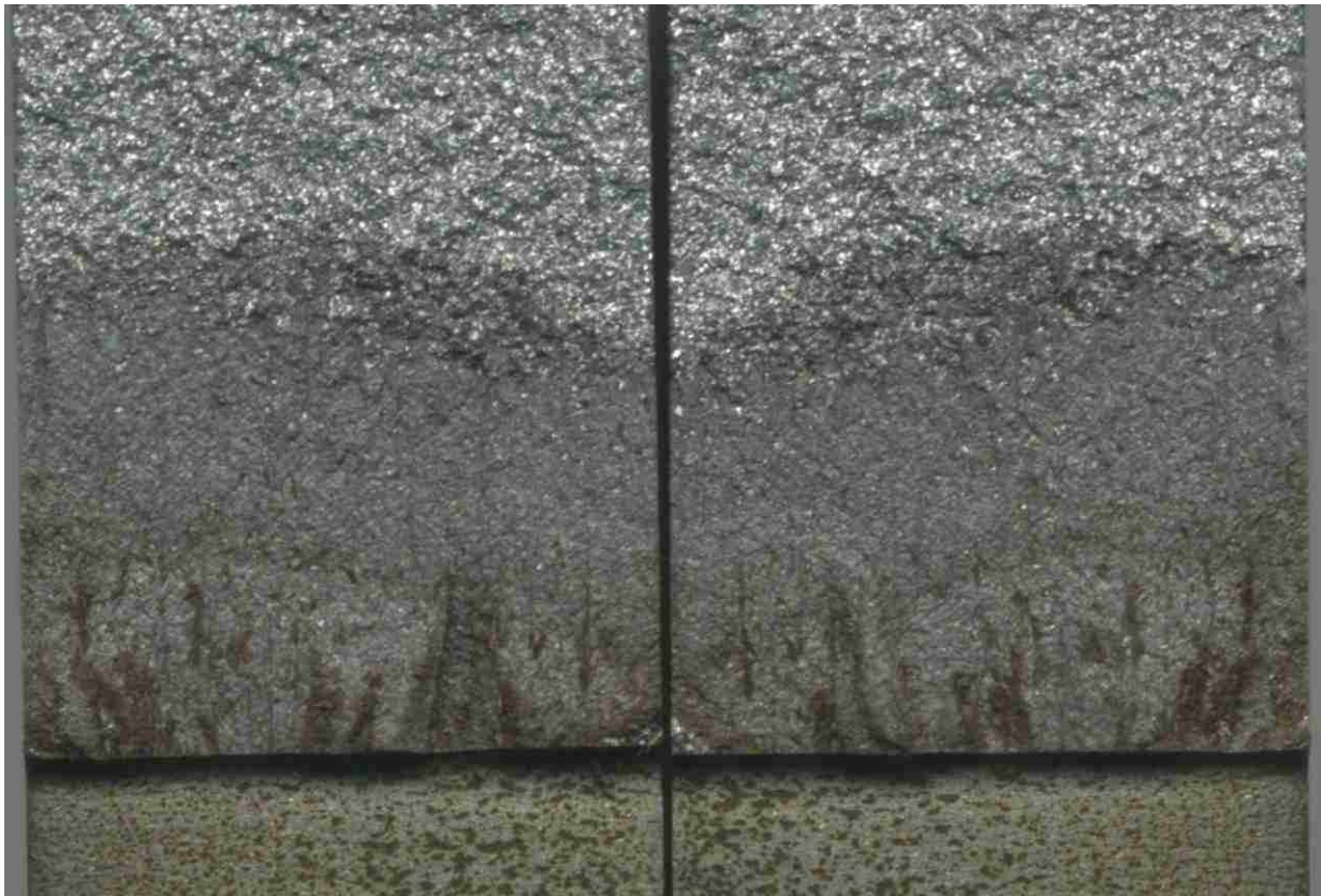
Figure 75 – Fatigue/fracture surface for HH 3B tested at R=0.1 .
