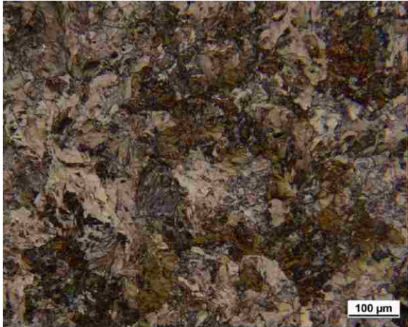
Figure 24 – LOM photomicrographs of Sample 4 from HAY84 rail as viewed at the mid length of the sample.
