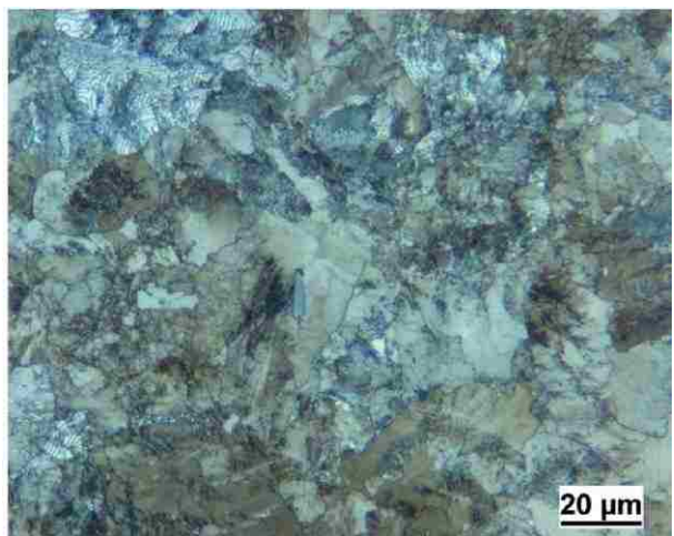
Figure 22 – LOM photomicrographs of Sample 4 from AHH rail as viewed at the mid length of the sample.
