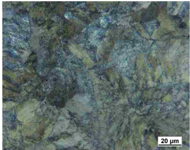
Figure 20 – LOM photomicrographs of Sample 4 from SS rail as viewed at the mid length of the sample.
