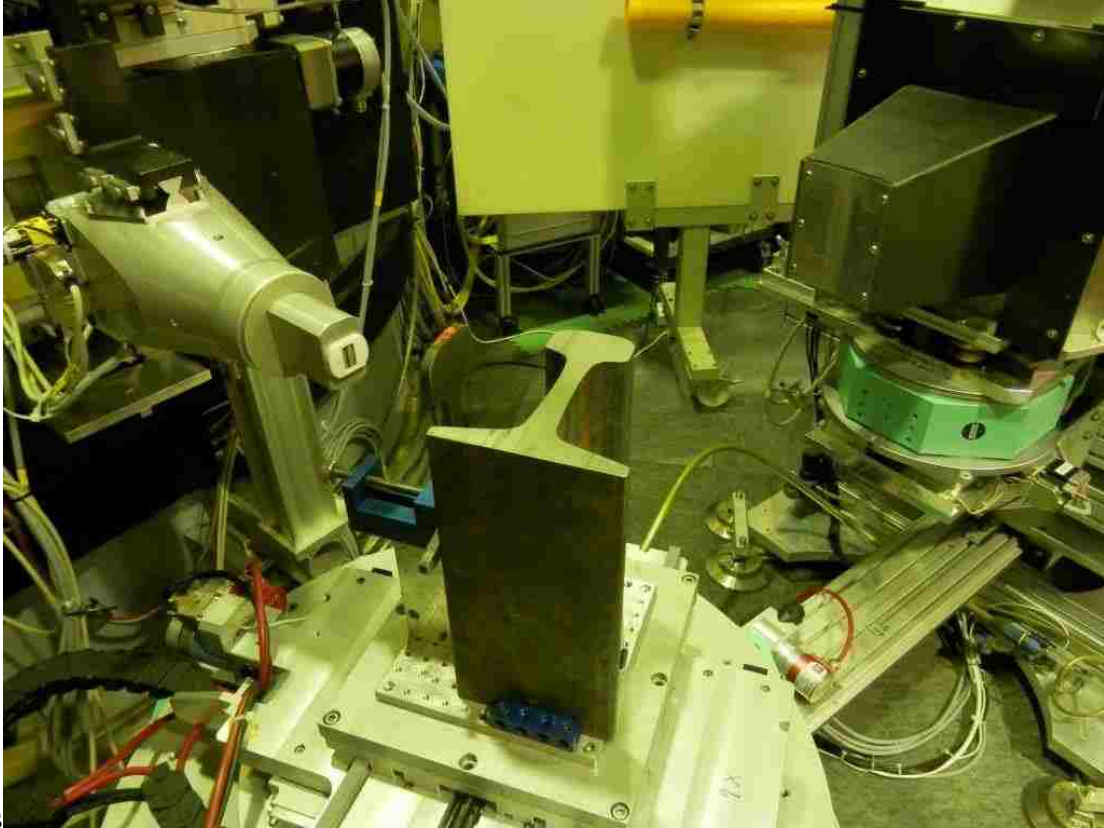
Figure 109 – Residual stress measurements on a 300 mm section of the AHH rail using the neutron source at Helmholtz-Zentrum Berlin (HZB).
