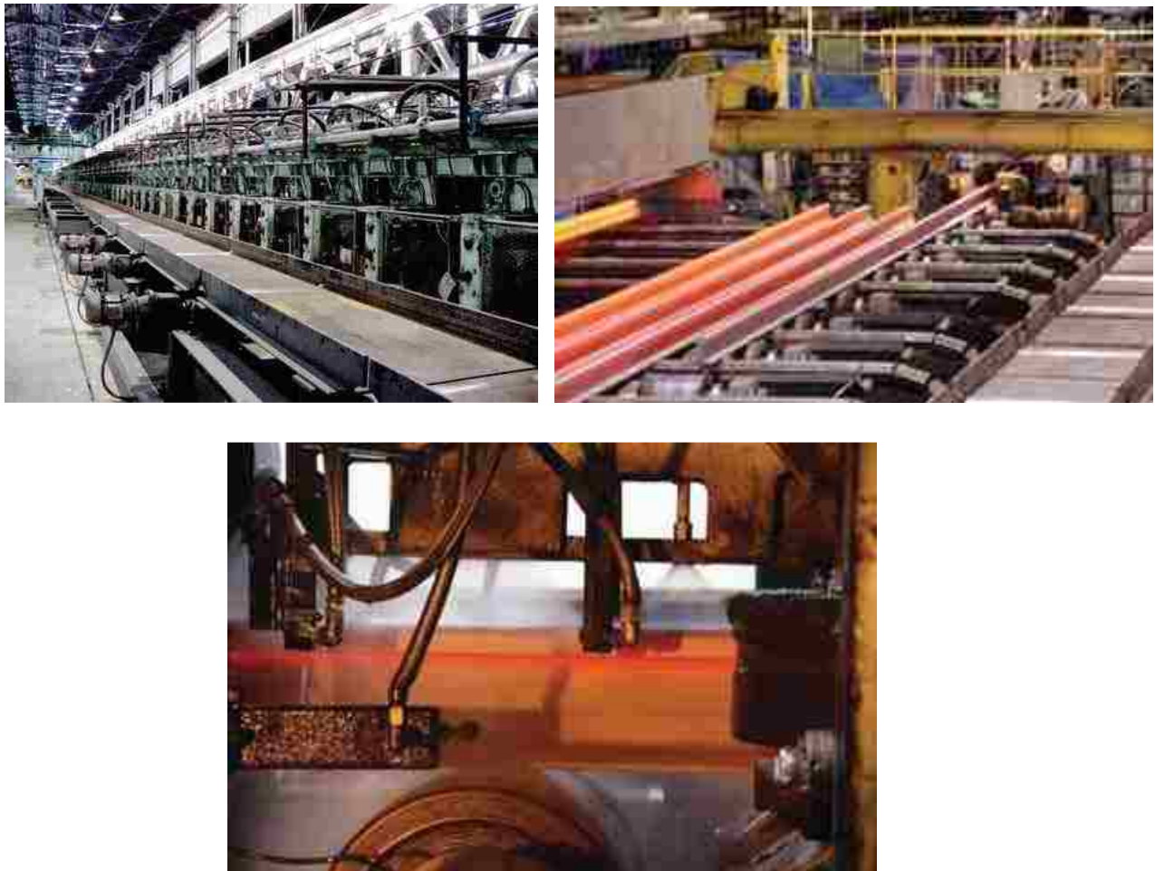
Figure 3 – Head hardening facility at ArcelorMittal, Steelton.
