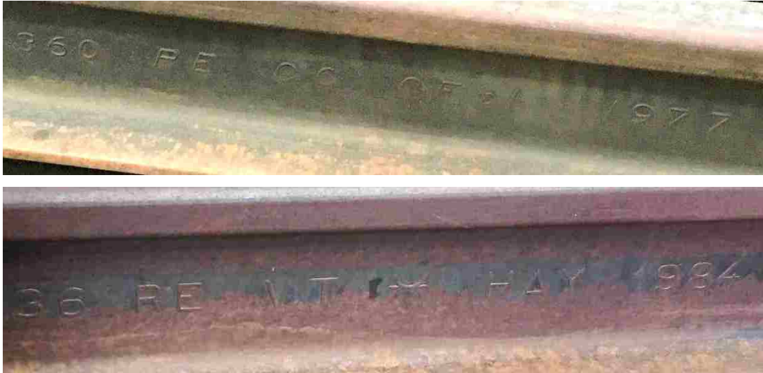
Figure 7 – Photographs of legacy rails, CF&I77 (top) and HAY84 (bottom), used to develop baseline data for comparisons with modern head hardened rails.
