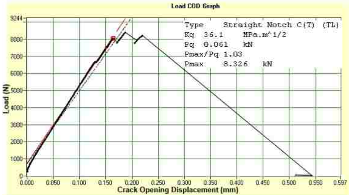
Figure 128 – Load vs COD for SS Rail Fracture Toughness Test.
