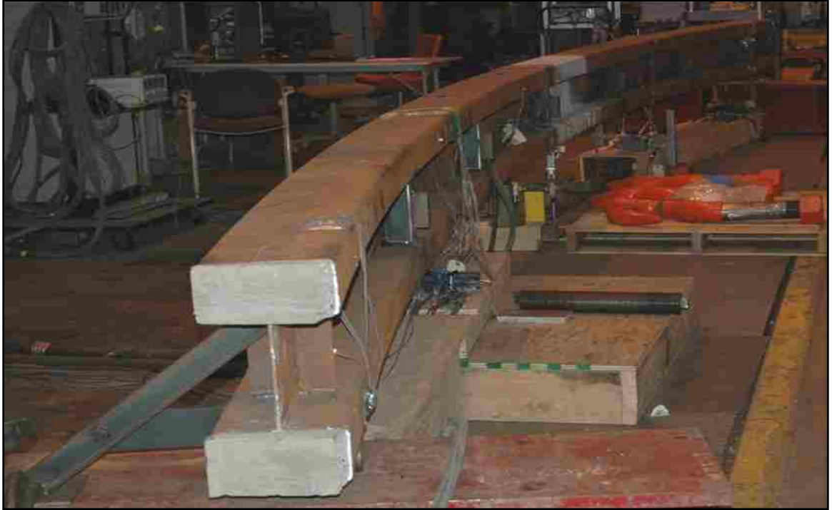
Figure 2.3 Curved TFG with hollow steel tube flanges and concrete infilled ends (Putnam, 2010)
