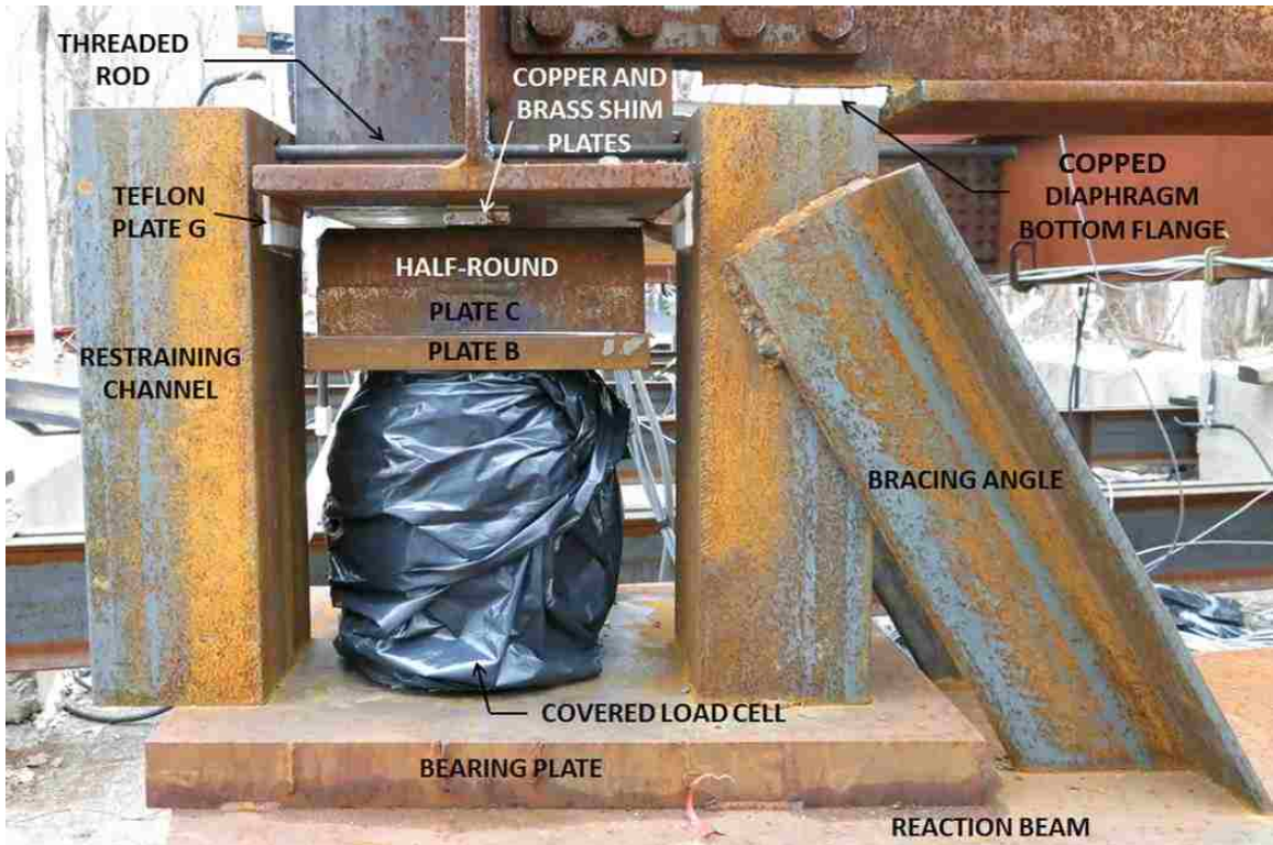
Figure 4.9 Photograph of G1E including radial restraining structure looking in circumferential direction
