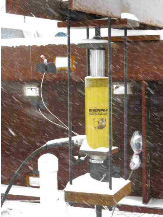
(a) Jack stroke before re-stroking
