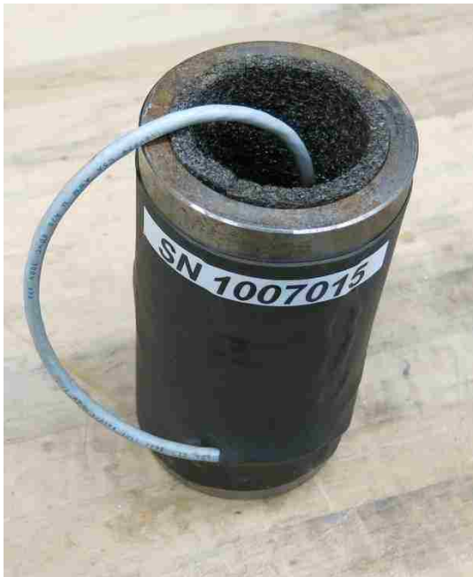
(c) Applied force through-hole load cell
