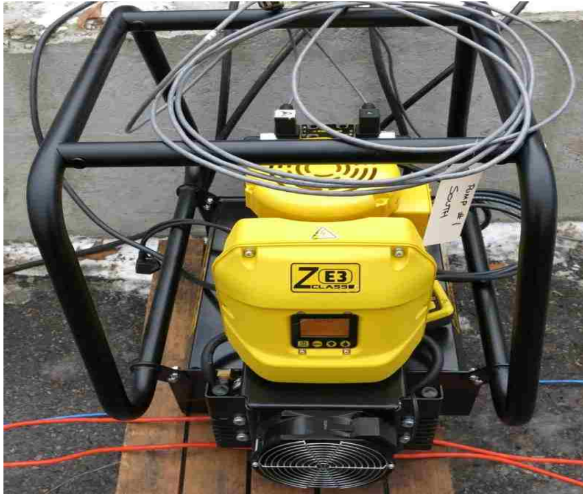
(a) ENERPAC ZE3 hydraulic electric pump
