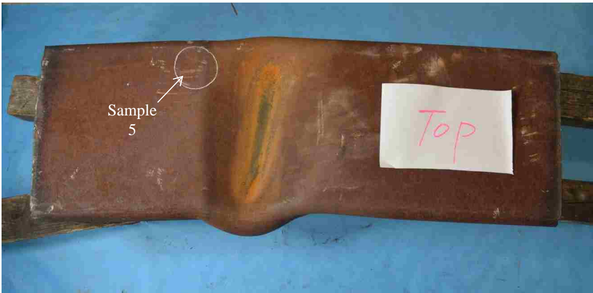
Figure 8.15 Buckled section looking from top
