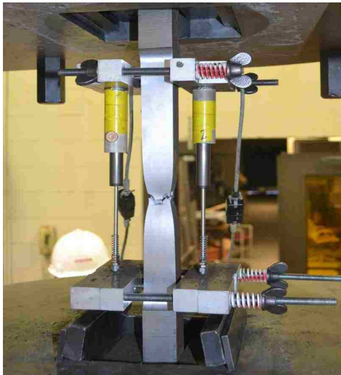
Figure 8.9 Tensile coupon after fracture
