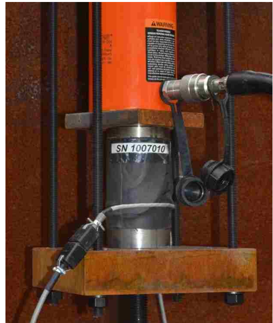
(d) Applied through-hole load cell in loading rod assembly
