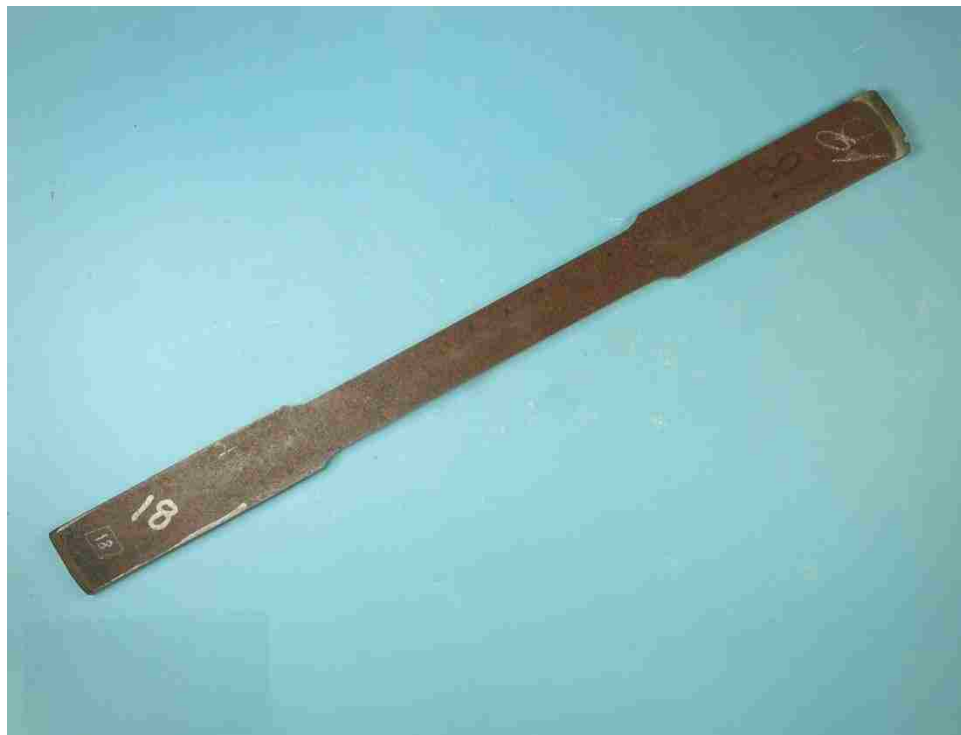
Figure 8.7 Plan view of typical tensile coupon
