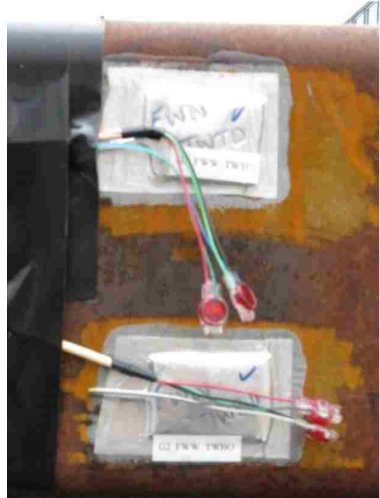
(b) Uniaxial strain gages on girder tube
