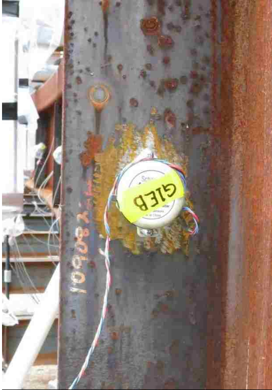
(a) Inclinometer attached to stiffener to measure test specimen rotation in radial plane
