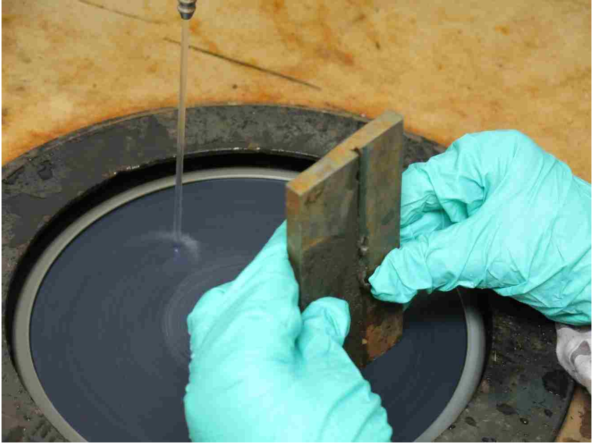
Figure 8.18 Grinding process during the metallography
