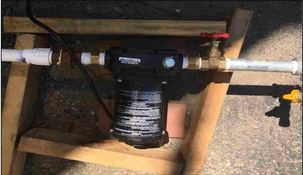
Figure 3.1: Wayne Self-Priming Cast Iron Portable Transfer Water Pump: The pump boosts line pressure up to 50 PSI, has a motor speed of 7500 RPM, and gives a flow rate of 1,450 GPH.
