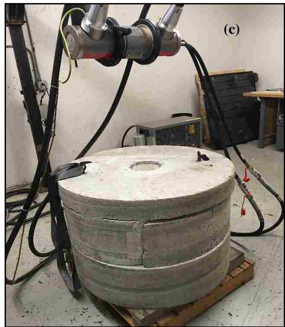
Figure 5.2 - Radiographic imaging: (a) shielding block assembly geometry (Keller & Pessiki, 2015), (b) shielding block assembly before installing the removable wall panel, and (c) final test configuration.
