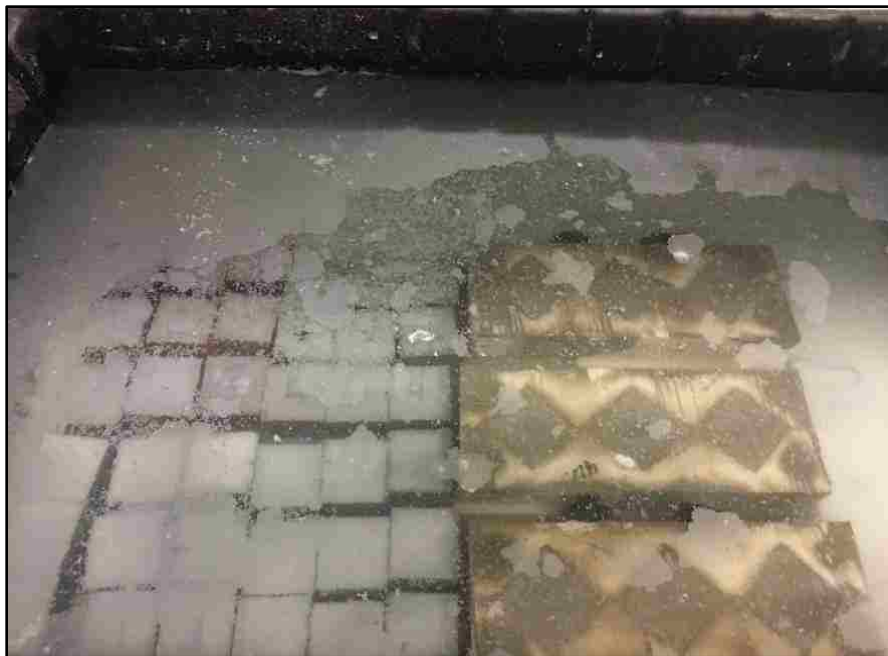
Figure 3.4 - Photograph of specimens immersed in a lime-saturated water bath for curing.
