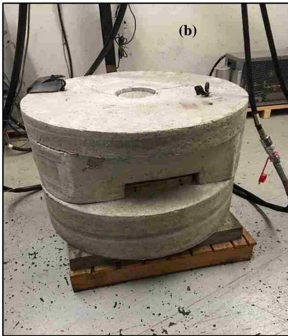
Figure 5.2 - Radiographic imaging: (a) shielding block assembly geometry (Keller & Pessiki, 2015), (b) shielding block assembly before installing the removable wall panel, and (c) final test configuration.
