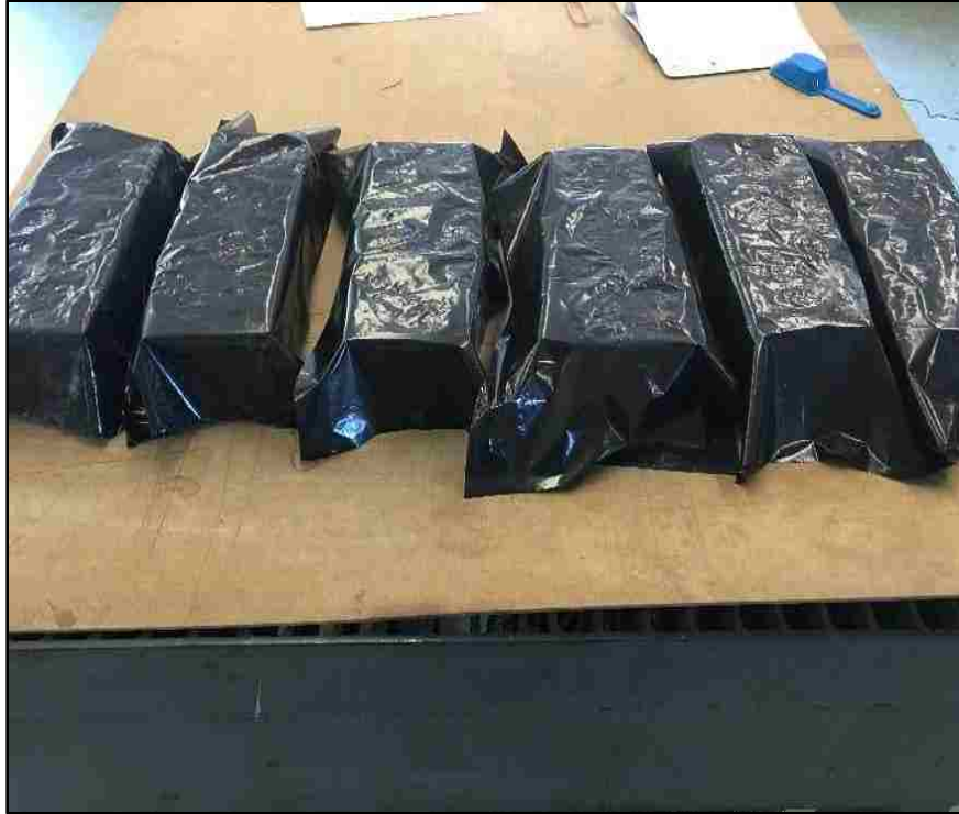
Figure 3.3 - Photograph of grout specimens covered with wet plastic sheeting prior to wet-curing.
