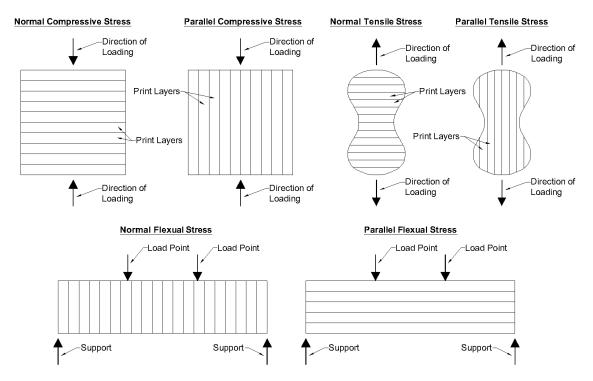
Figure 2: Printed Specimens Loading Orientations
