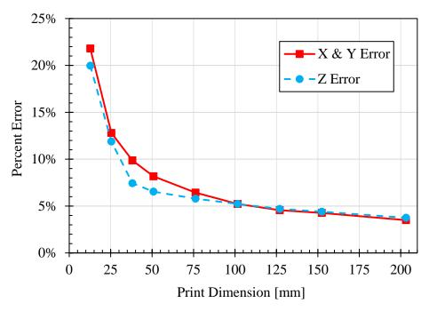
Figure 4: Printer Bleed Correlation with Print Dimension
