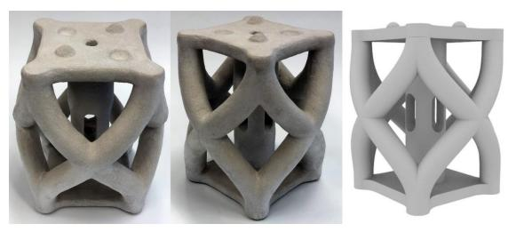
Figure 6: Geometric Sample Print, Front View (Left), Side View (Center), STL (Right)
