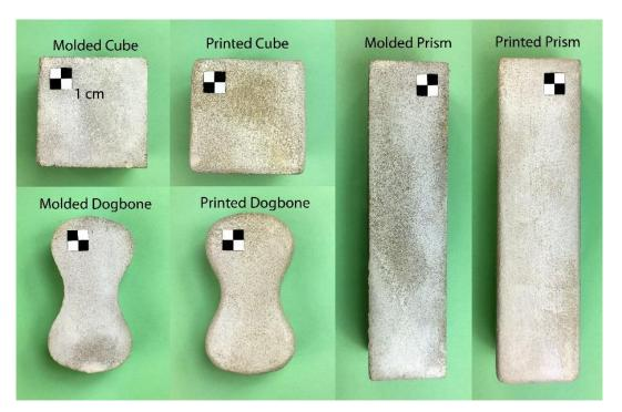
Figure 3: Printed and Molded Test Specimens
