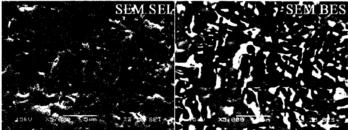
Figure 2.10 Comparison of SE and BE SEM images of (U_4Th_2Zr_9)H_{1.5} sample.
