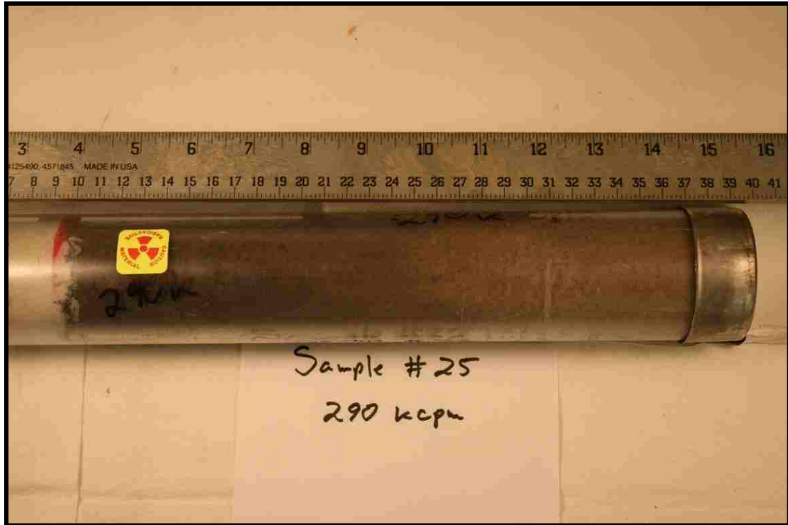
Figure 8. Picture of a typical core. The white material on the left side is expanding foam used to fill headspace prior to shipping. A plastic cap (red) is used to isolate the soil from the foam. Steel caps were used to seal both ends of the core.
