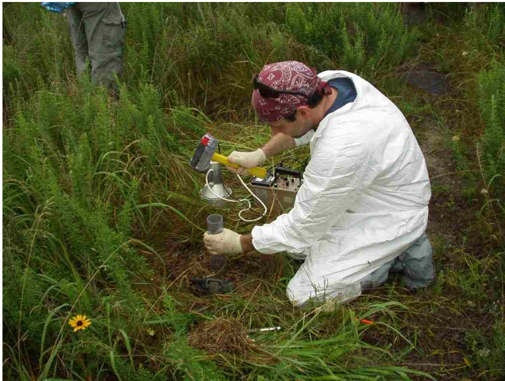
Figure 7. Obtaining a core containing a WGPu hot particle. The 51 mm diameter PVC tube was manually driven into the ground to collect the core. The FIDLER used to locate the ^{241}\text{Am} signal from the hot particle is located in the background.
