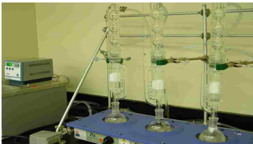
Figure 35: Soxhlet apparatus for corrosion experiments. Cellulose thimbles seen in chamber to suspend sample above water volume.
