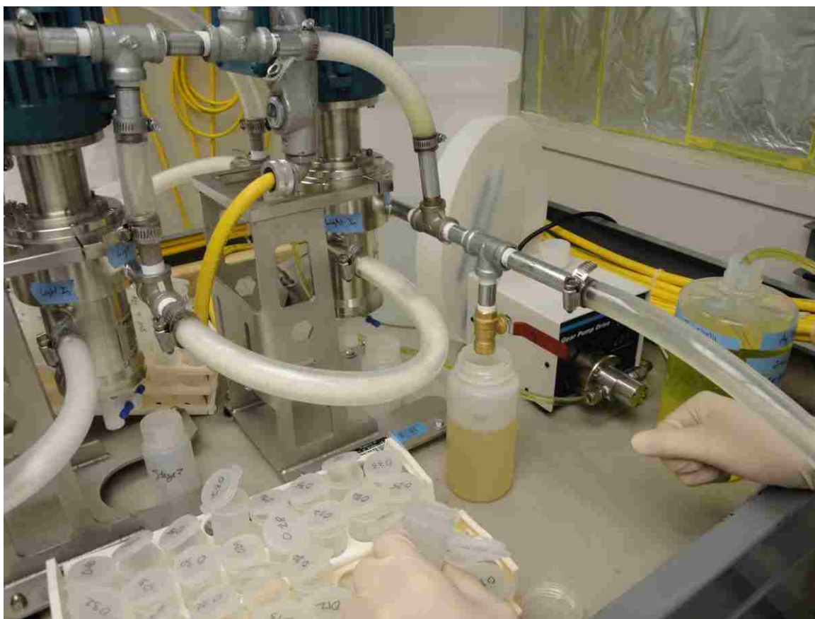
Figure 37: Foaming in organic interstage tubing
