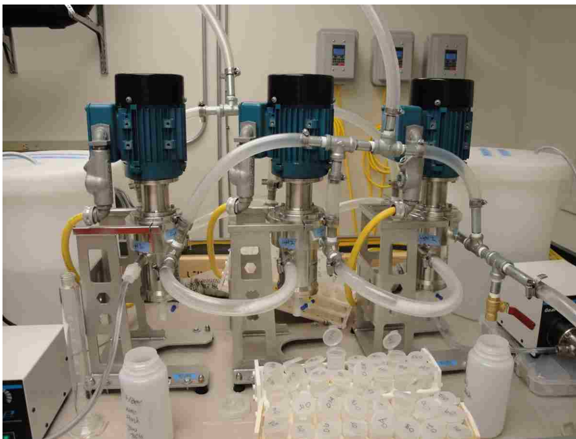
Figure 33: Bench of 3 V-02 contactors at UNLV
