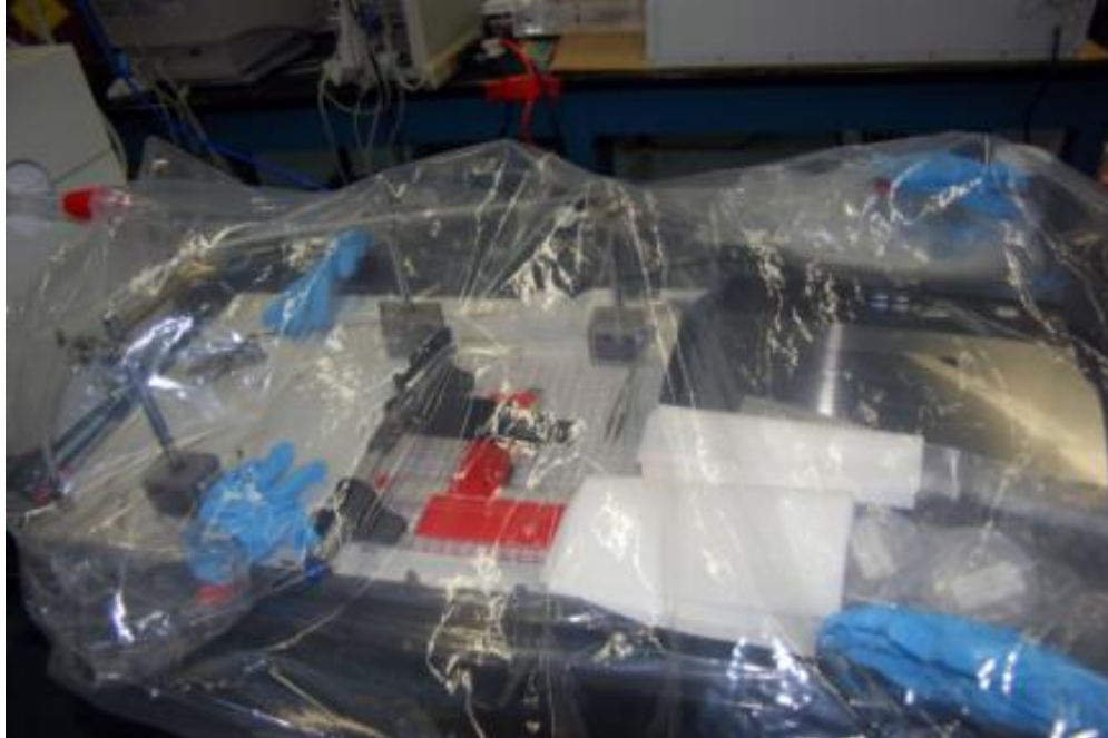
Figure 4.2: Furnace 1 glovebag setup.
