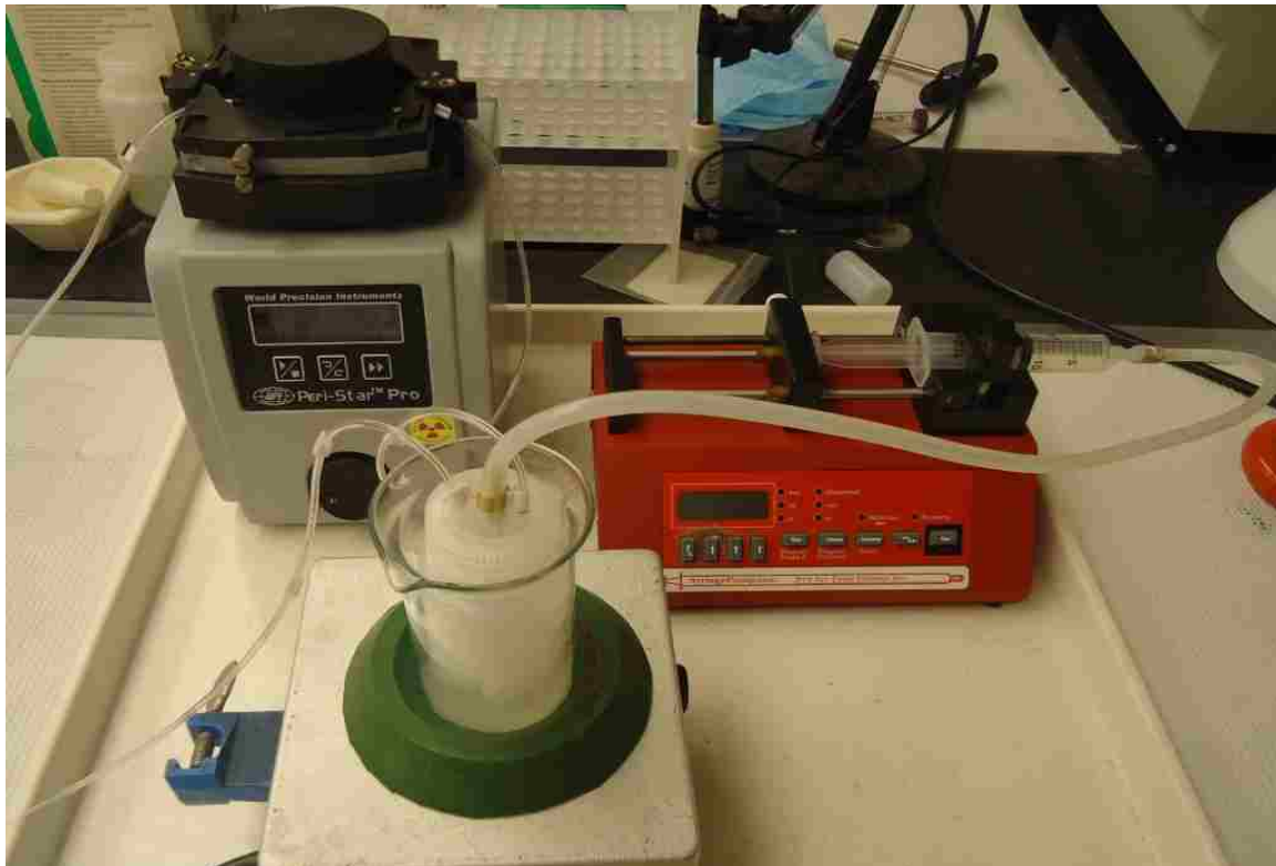
Figure 11 - Spectrophotometric titration apparatus. Syringe Pump (Upper Right) delivers titrant to sample cup (foreground) on a stir plate. Peristaltic Pump (Upper Left) recirculates sample through flow through cuvette (not shown).
