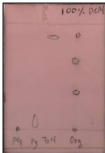
Figure 19. TLC results from tosylation of 2',3'-O-isopropylidenguanosine after overnight reaction. (PG: 2',3'-O-isopropylidenguanosine, Py: pyridine, TsCl: p -toluenesulfonyl chloride, Org: organic layer (ethyl acetate) after extraction, Eluent: 100 % dichloromethane)
