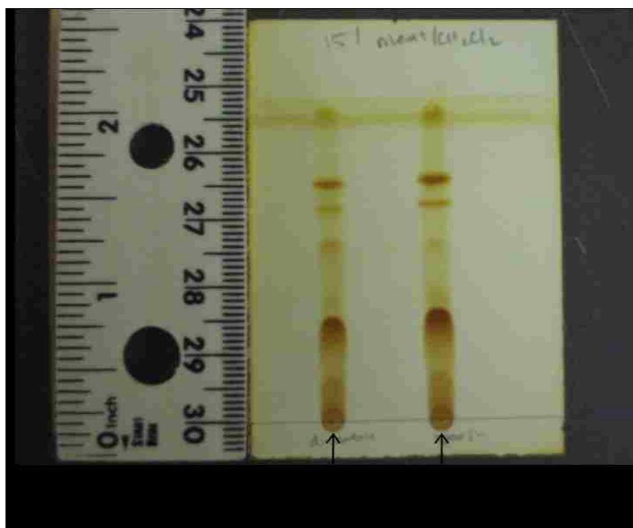
Figure 19. TLC plate of d-lenolate & Spanish Olive Leaf Extract developed in 15% MeOH/CH 2 Cl 2 solution.
