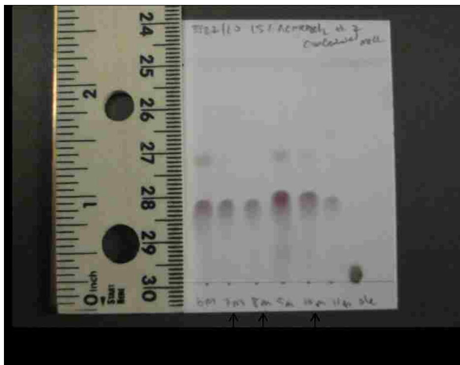
Figure 18. TLC plate of samples M7, M8, & M11 developed in 15% ACN/CH 2 Cl 2 solution.
