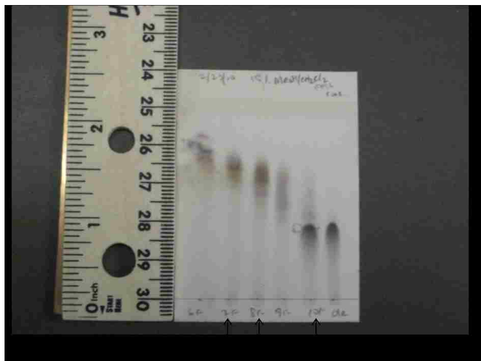
Figure 16. TLC plate of samples B7, B8 & B10 developed in 15% MeOH/CH 2 Cl 2 solution.
