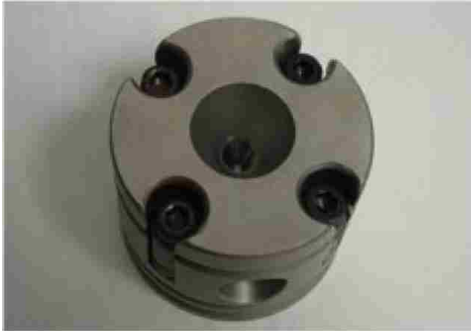
Figure 8. Princeton symmetric type diamond anvil cell (DAC)
