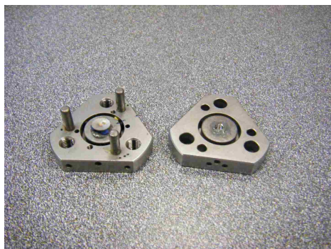
Figure 6. A Merrill-Bassett 3-pinned DAC was used for the Raman measurements.
