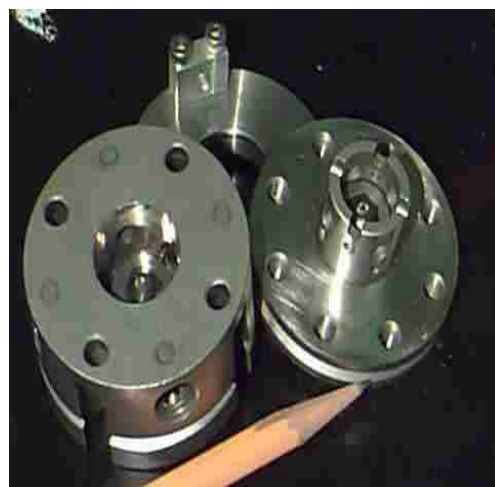
Figure 7. Symmetric type cell was used for the IR measurements.
